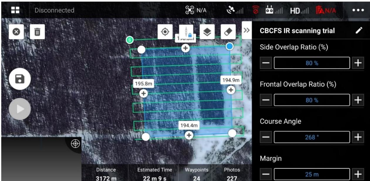
**Figure 6. Image capture parameters and the flight path plotted with DJI Pilot for the 4-ha scan area.**
