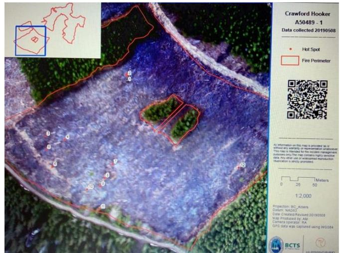
**Figure 4. Hotspot map produced as the deliverable from infrared scanning mission.**
