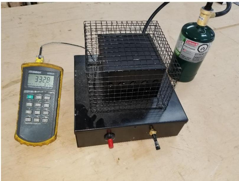
**Figure 5. Simulated hotspot used in detection trials.**
