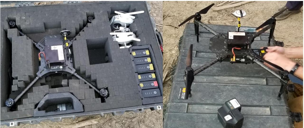
**Figure 2. The Matrice 100 packed in its hard case (left) and assembled (right) showing enhanced GPS antennae.**
