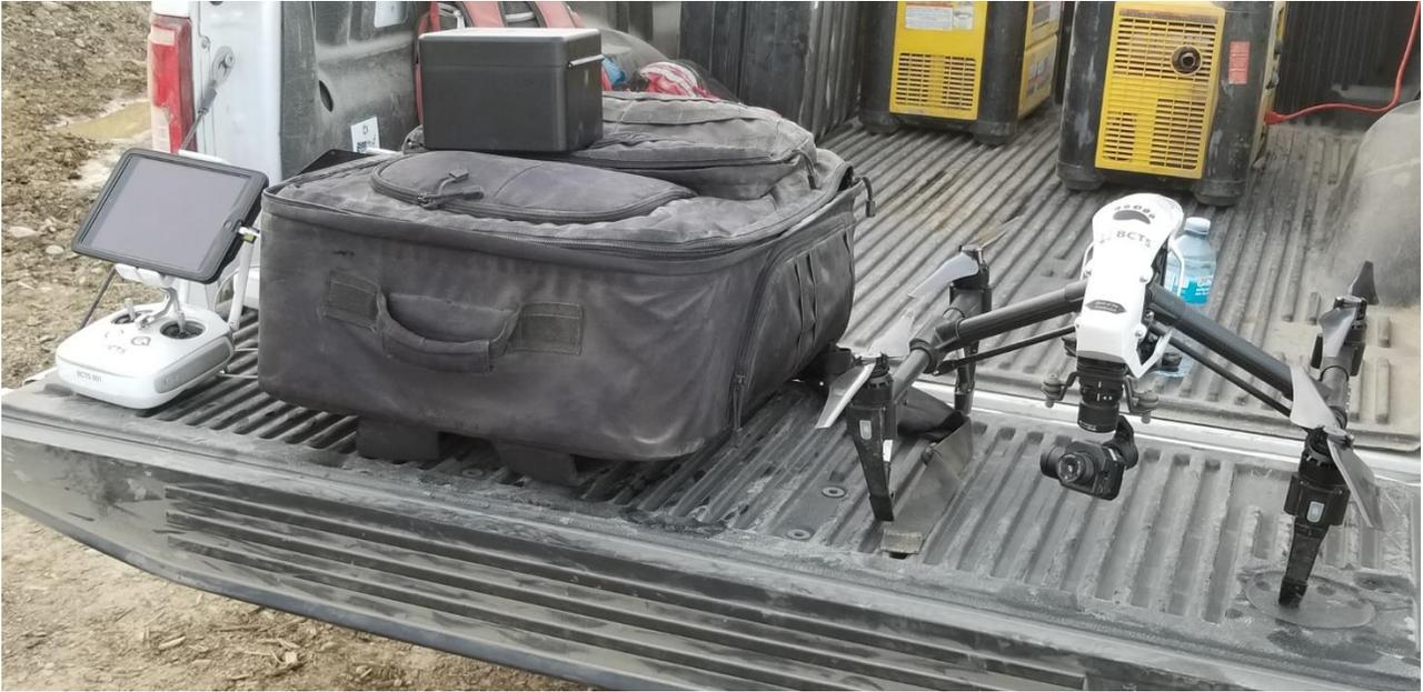
**Figure 1. Components of the DJI Inspire 1 Pro RPAS including aircraft, sensor, remote controller, and tablet.**
