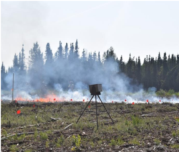
Figure 5. Coarse mulch subunit instrumented with array of flags to document rate of spread.
