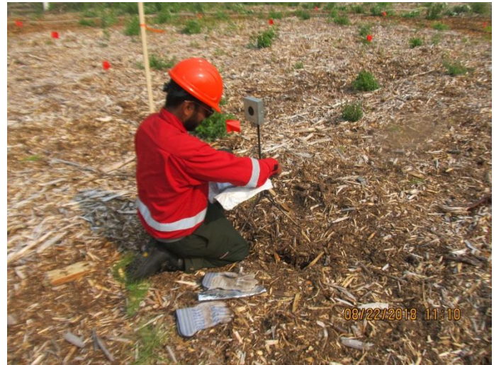
Figure 6. Installing heat flux sensors in the fine mulch fuel bed.
