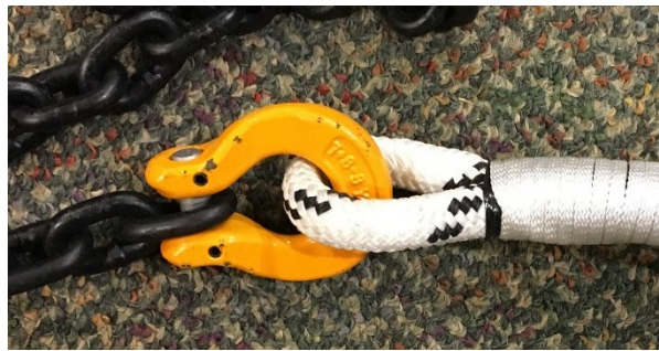
Figure 5. Yellow connector used to join the DT rope and chain
