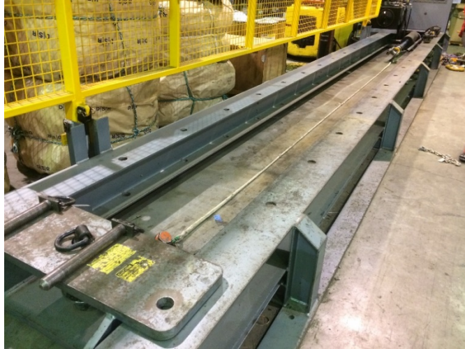
Figure 2. Rope in test machine
