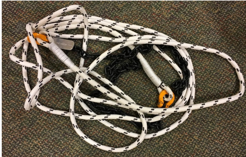
Figure 4. Log load wrapper made from DT rope.
