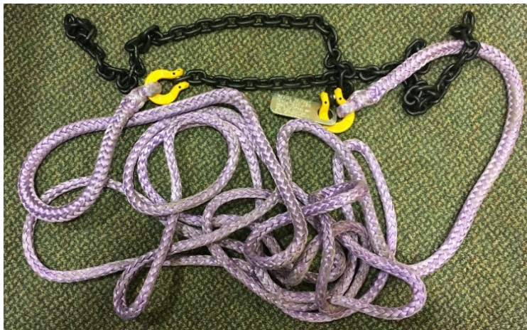
Figure 3. Log load wrapper made from 12.5 mm Plasma rope
