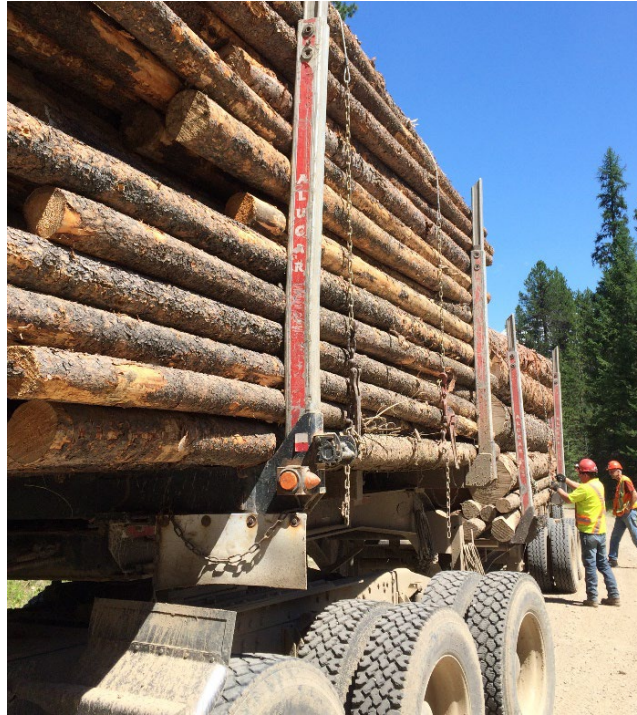
Figure 1. Load wrappers around log load
