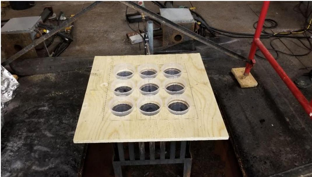
**Figure 6. Cup-and-grid method to measure coverage levels.**
