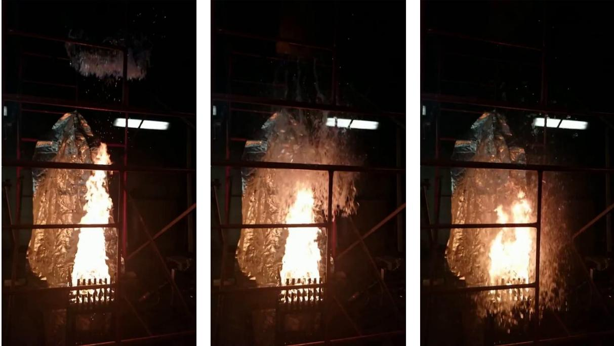
Figure 10. Flame immediately prior to suppression.
