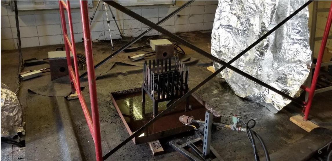
Figure 5. Catchment tray located beneath the crib holder.
