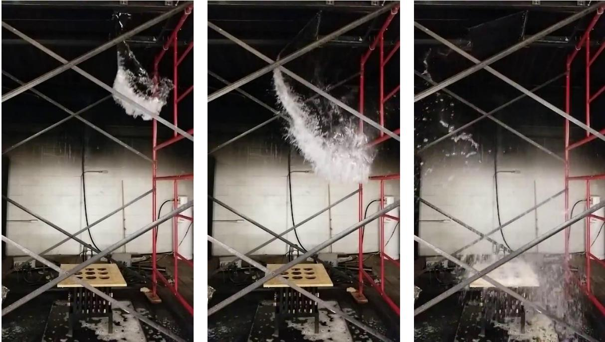
Figure 21. Drop dynamics of WD881C at 0.3% (left to right).
