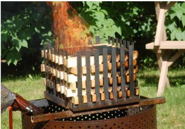
Figure 1. A preliminary burn of a test crib with six slat layers. The crib top is absent in this image.
