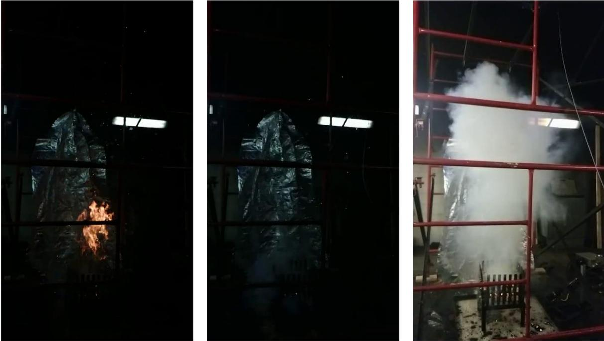
Figure 11. Resulting flame immediately after suppression.
