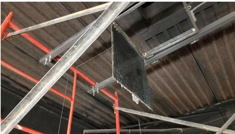
Figure 4. Tank with the bottom open to allow suppressants to drop on a burning crib.
