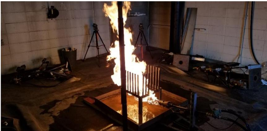
Figure 2. Crib holder without the wooden slats (center) and a torch applying propane.
