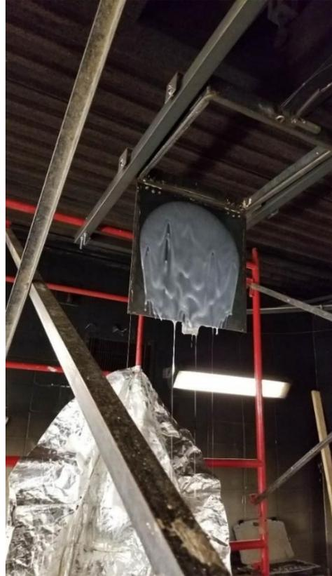
Figure 19. Firewall II at 2% stuck to the drop tank door.
