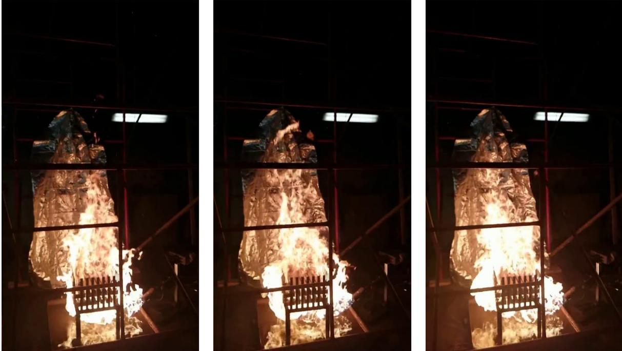
Figure 8. Crib ignition using torch.
