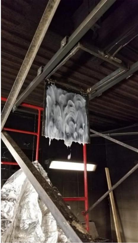
Figure 18. Thermo-Gel at 2% stuck to the drop tank door.
