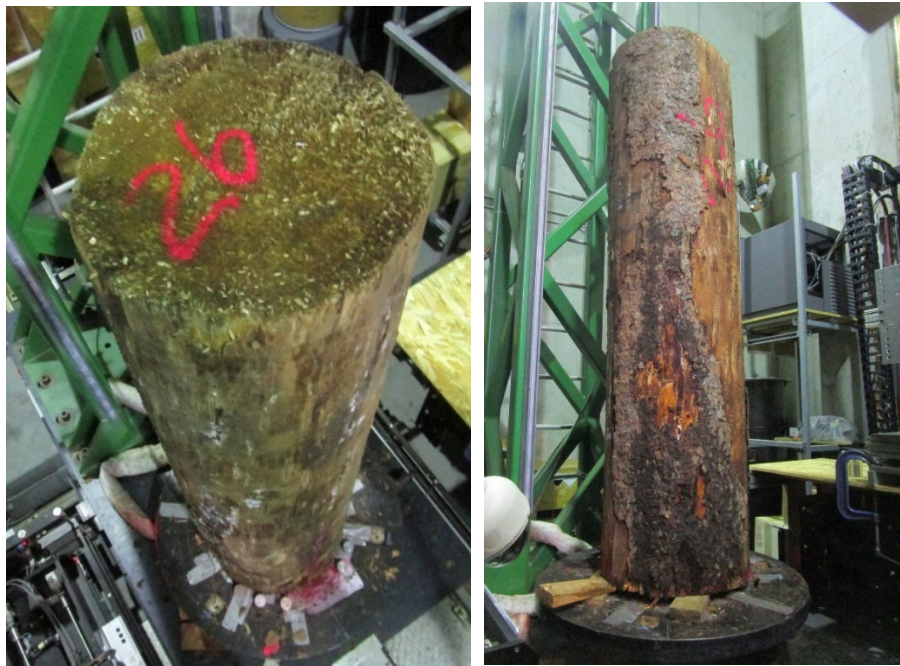
Figure 2. Examples of log set up in the CT bay to be scanned
