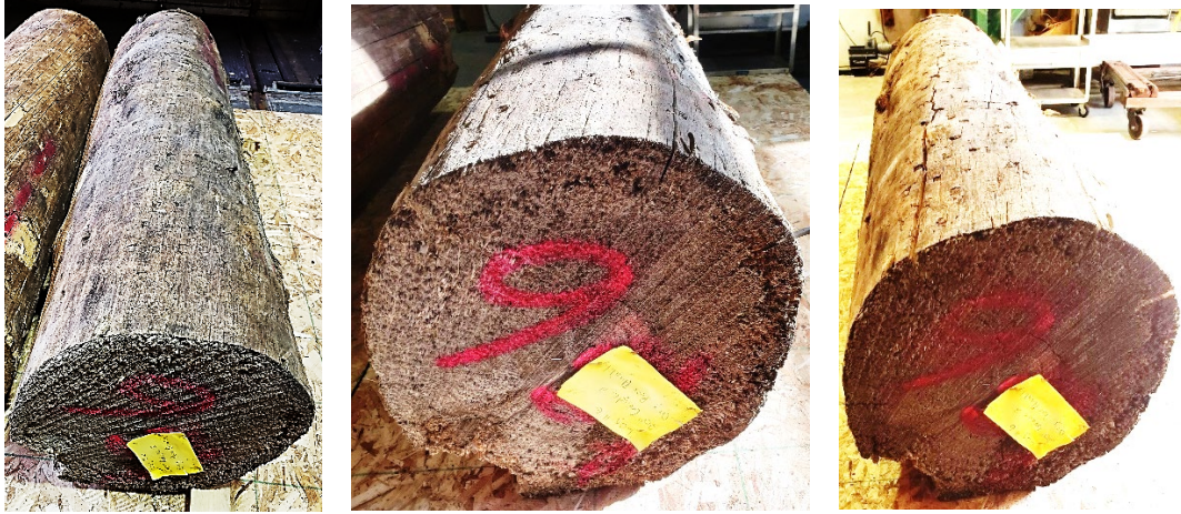
Figure 8. Log 6 before (left) and after (middle) warming and one month stay in the lab(right)
