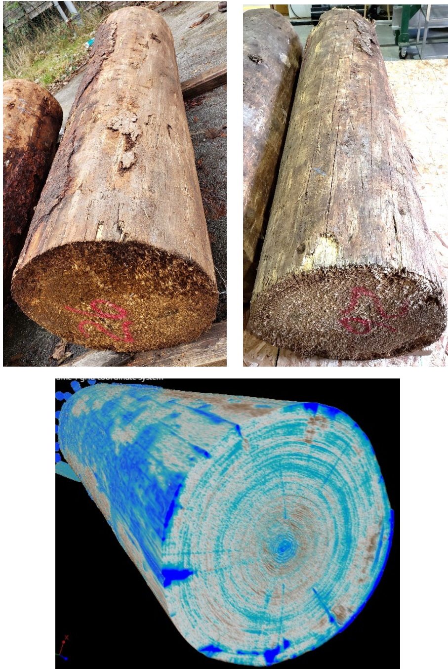
Figure 5. Log 26 rain-soaked in yard (left), in lab before warming (right), 3D CT image (bottom)
