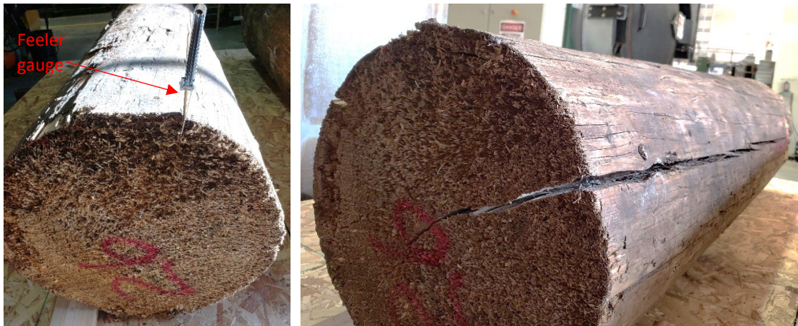
Figure 6. Log 26 after warming (left) and one month in the lab with similar temperature and RH (right)
