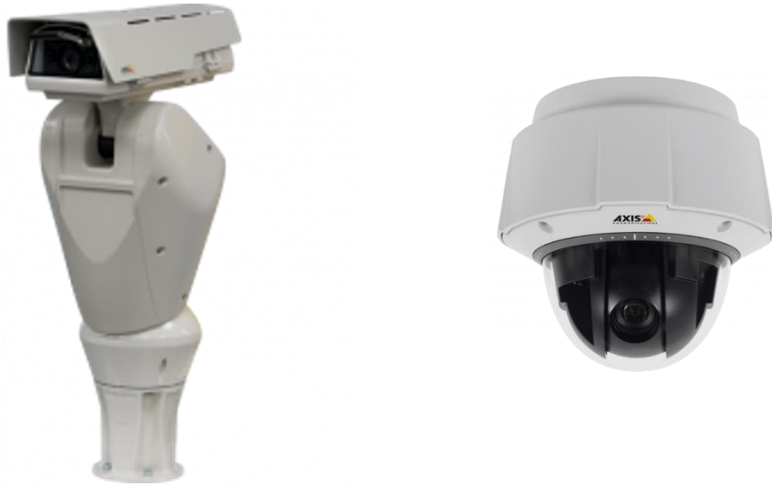
Figure 4. A non-dome style PTZ camera on the left and a dome style PTZ camera on the right. Source: axis.com
