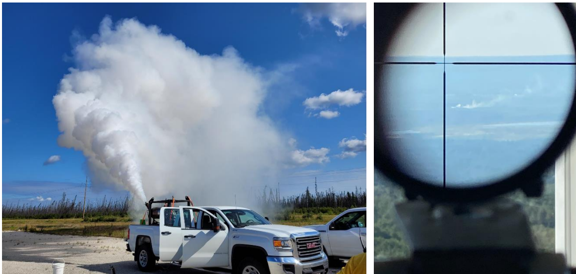
Figure 1. A smoke generator producing artificial smoke (left). An image of the same smoke captured by the lookout observer through a fire finder at a range of 23 kms (right).
