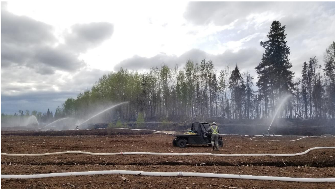
Figure 37. West-bound 4-inch line, 250-meters in length, containing 4 water cannons.
