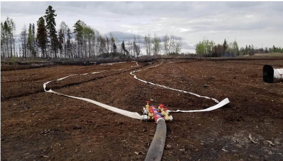
Figure 2. Mixed system with a 6-inch main line and 4-inch off-shoots.
