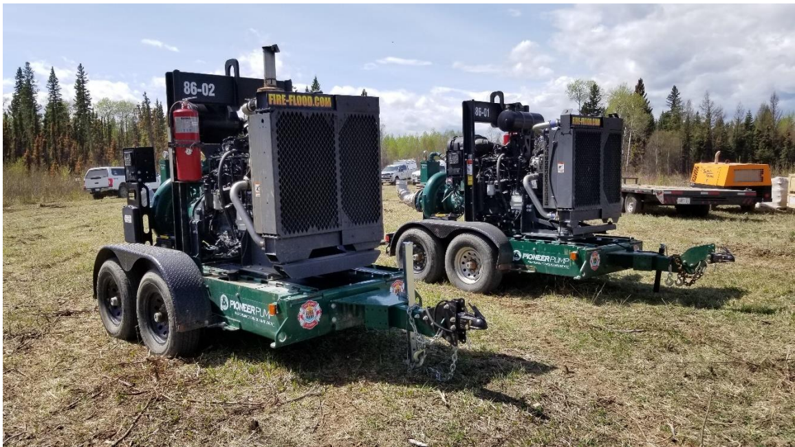
Figure 15. Two 335 HP pumps were used for water delivery operations. Only one pump was used on Day 1.
