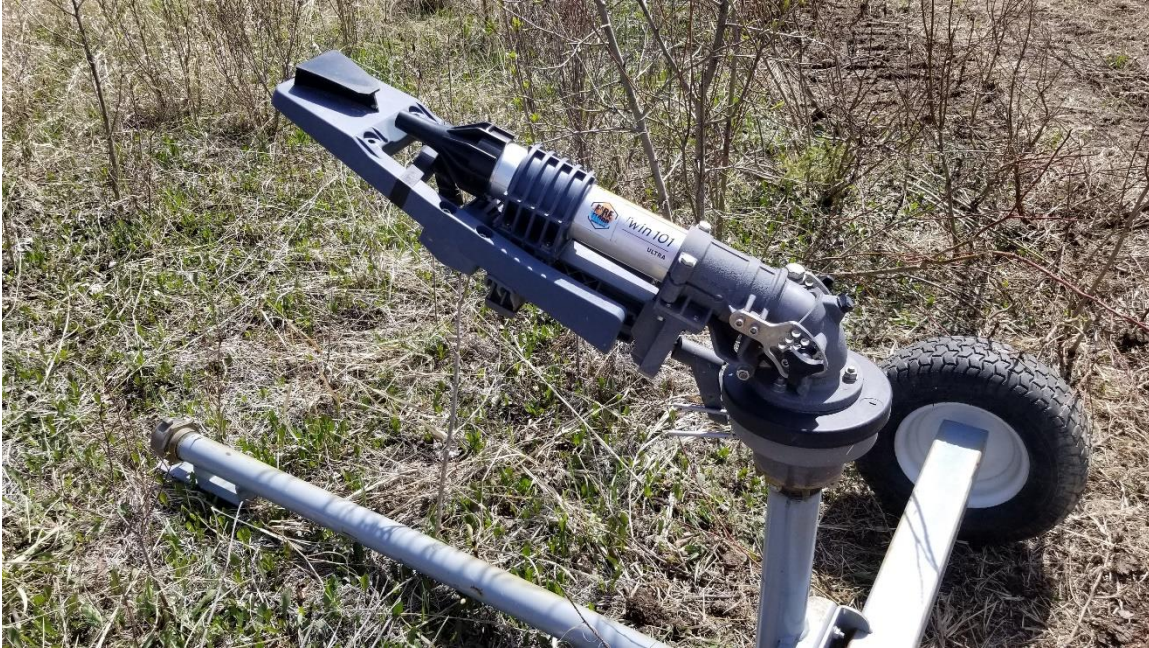
Figure 18. Water cannons used in water delivery operations.
