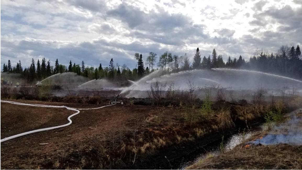
Figure 29. 4-inch systems with water cannons working on Hotspot 1.
