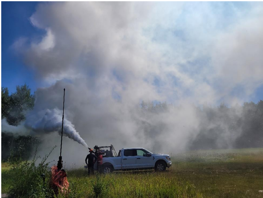
Figure 4. The Curtis Dyna-Fog 1200 smoke generator.
