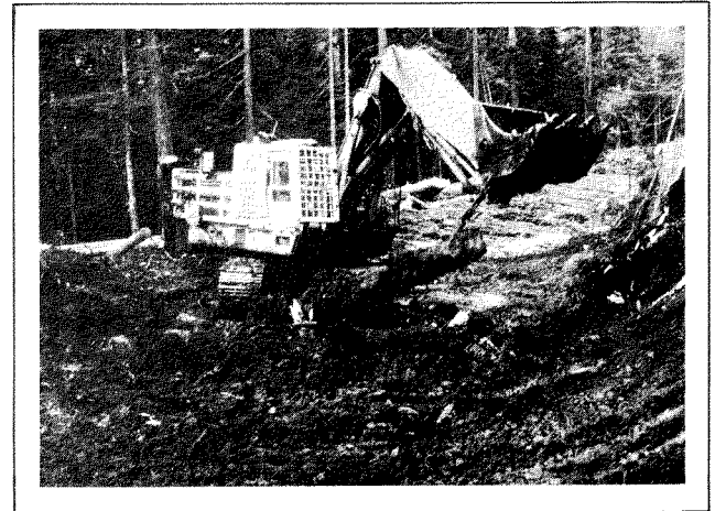
Figure 4-c. Hydraulic shovel moving ahead on shovel mats
