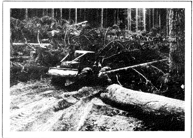
Figure 2-a. Timberjack 404 skidder yarding logs on the right-of-way
