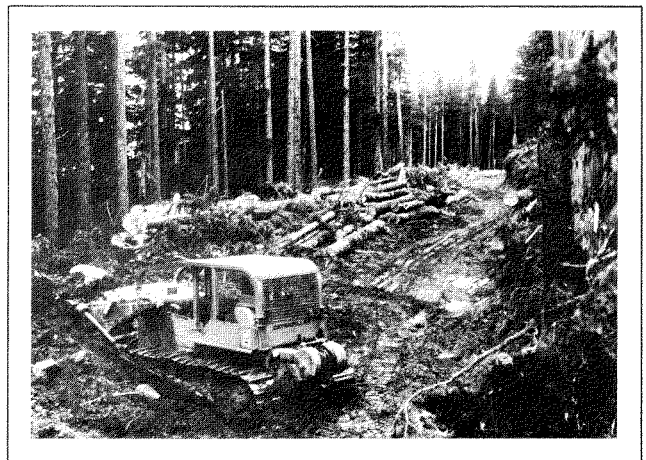
Figure 2-b. Bulldozer preparing a log deck
