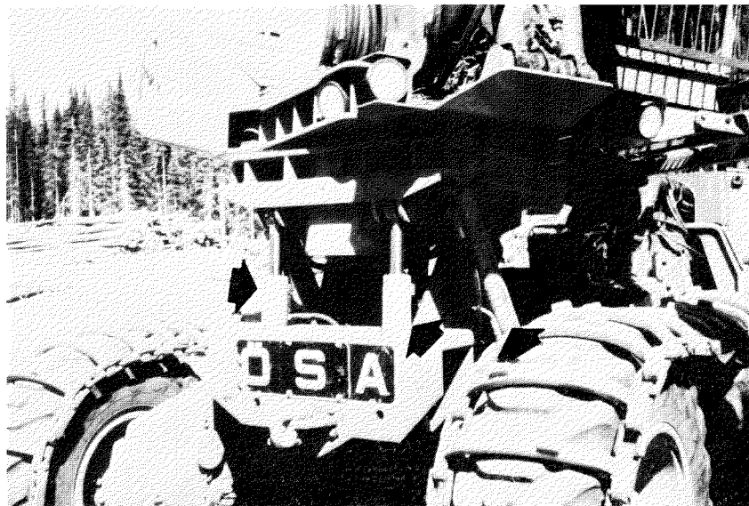
Figure C. Closeup view of turntable levelling system. Arrows indicate hydraulic cylinders used to achieve levelling of cab and turntable up to 30%.
