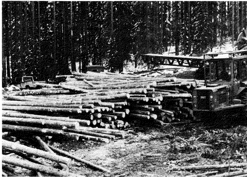
Figure K. Pile of processed logs at landing after single pass by processor. Note the excellent limbing quality.
