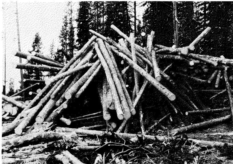
Figure L. Pile of processed logs after multiple passes in a congested landing. Limbing quality is excellent, but butt and top logs are mixed and piling quality is poor.
