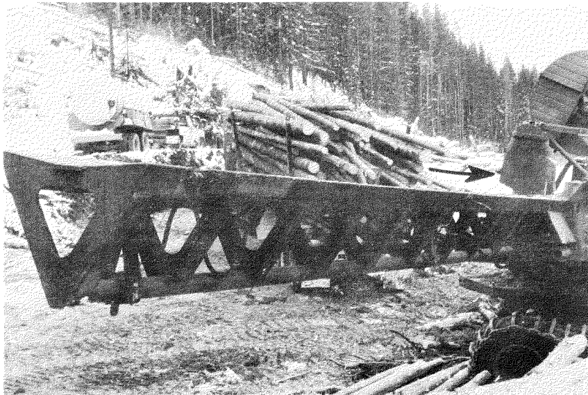
Figure F. Outfeed tray for processor. Arrow indicates rubber flap which activates the log-length measuring device.
