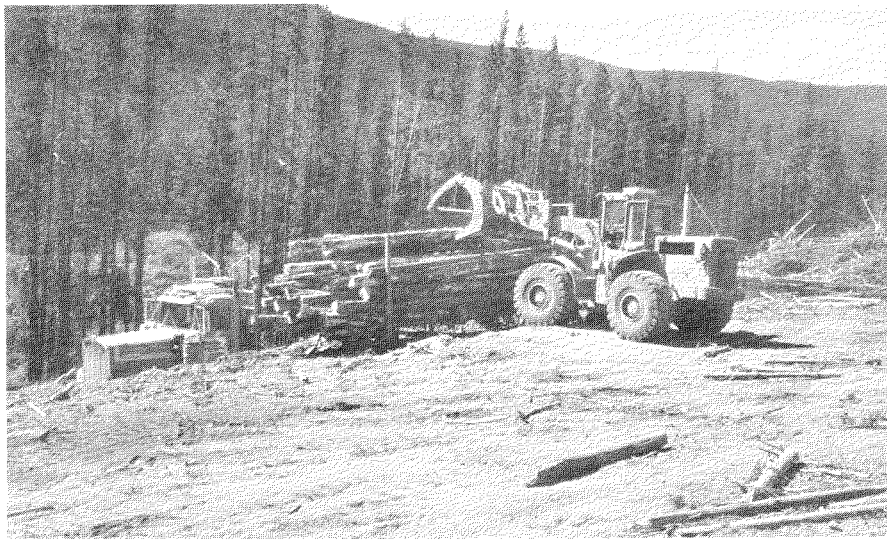
FIGURE G. Loading highway truck at bush landing-- Conventional System, summer phase
