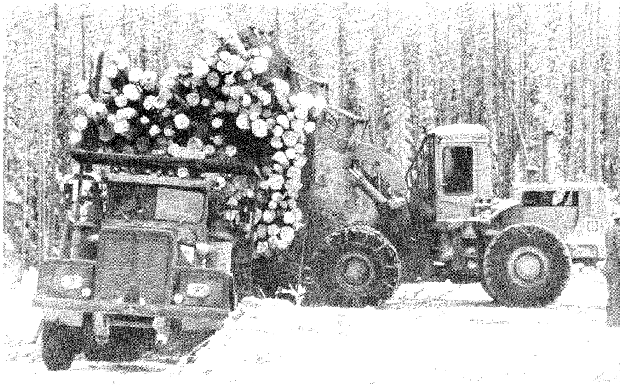
FIGURE F. Loading off-highway truck at bush landing-- Central Processing Yard System, winter phase
