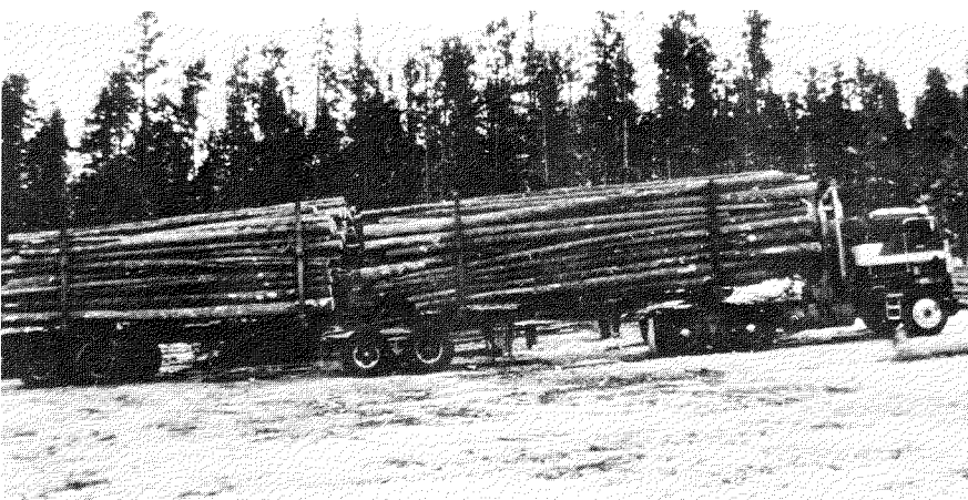
FIGURE 5. 7 Axle - 'B' Train, 2 Semi-Trailers
