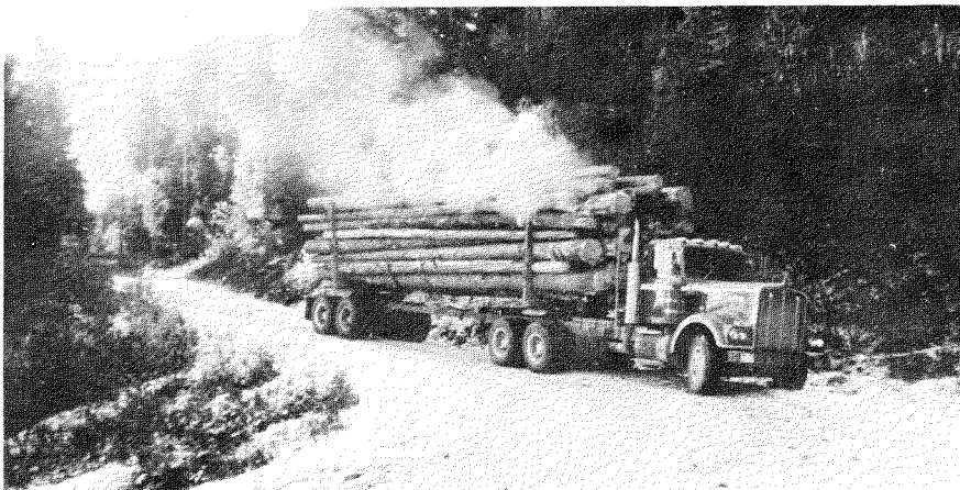
FIGURE 3. 5 Axle - Standard Pole Trailer
