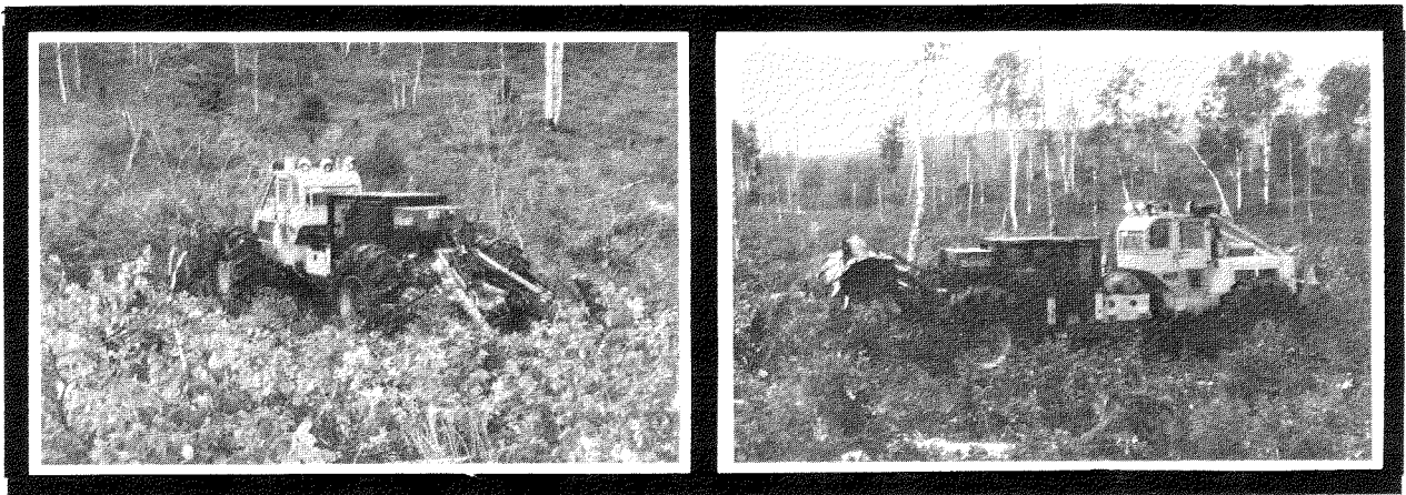
Figure 9. Operating positions of discs. Left: Donaren scarifying with discs lowered. Right: Manoeuvring in site between passes with discs raised.
