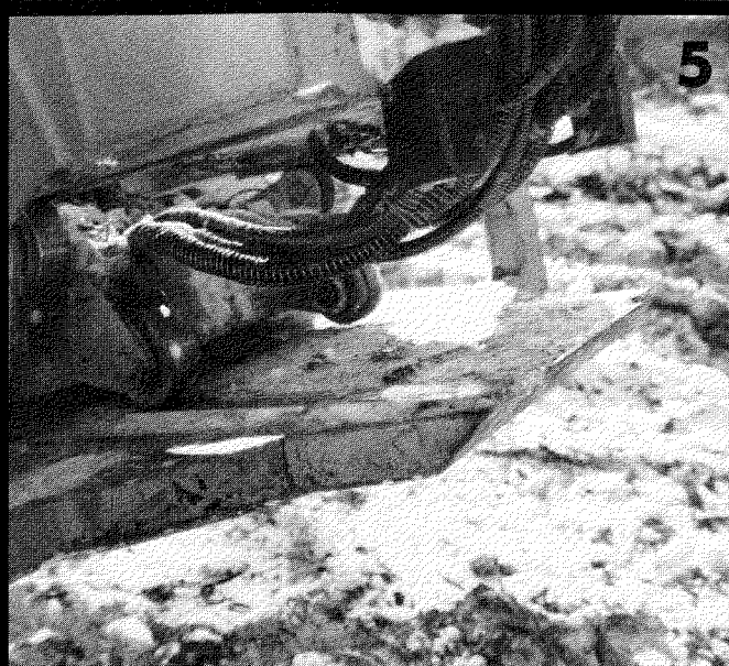
Fig. 6. Harriicana circ. saw head on JD693 at United-Sawmill, Hearst, Ont.; 1: felling and unching in a black spruce stand; 2: arrow shows location of the second oil cooler; 3: Harriicana circ. saw head after 8 months of use; 4 & 5: hydraulic hose failure at the back of the felling head was a major cause of repair downtime. This problem has been eliminated on the new design (see Fig. 8); 6: trees up to 50 cm (20 in) butt diameter were felled with the new design (see Fig. 8); 6: trees up to 50 cm (20 in) butt diameter were felled with virtually no butt damage. Note the rough, frayed surface made by the saw.
