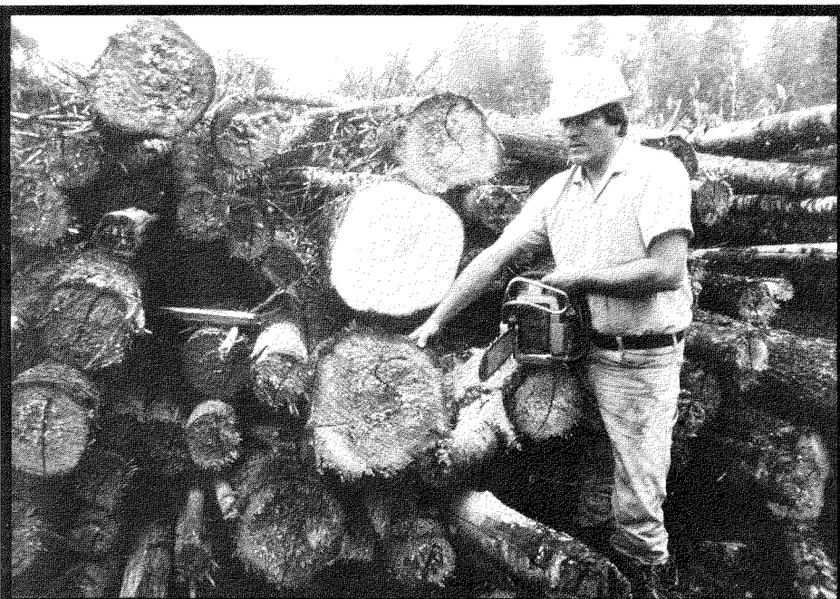
Fig. 3. The Koehring disc saw (similar to the Harricana and Lokomo units) normally produces a rough, frayed surface. This may cause difficulty in determining the extent of butt rot for bucking or scaling purposes. The log in the centre has been freshly cut with a chain saw.
