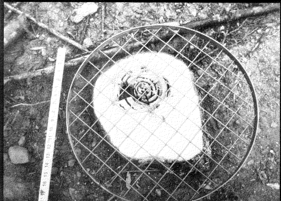
Fig. 4. Butt damage studies of trees felled by the K2FF's disc head were made using the "Bicycle Wheel" method. It showed that the rough, frayed surface (see Fig. 3) was superficial. On most trees there was no evidence of butt splitting or other damage. Even trees with extensive butt rot, such as the one shown to the left, were undamaged. If this tree had been cut with a shear the butt section would probably have been crushed. (See Appendix A for the study results.)
