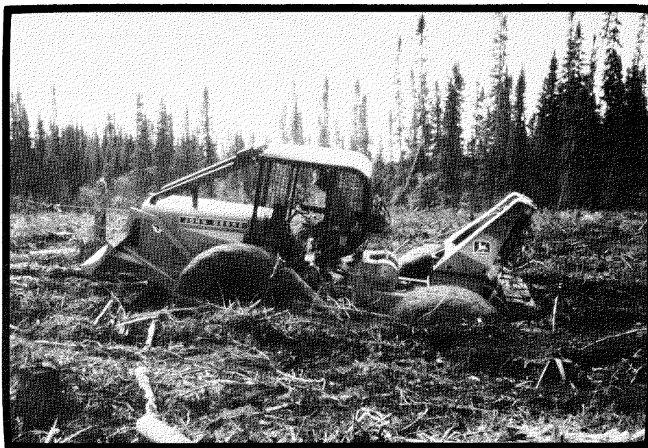
Figure 1. Excessive Sinkage with Conventional Tires.
