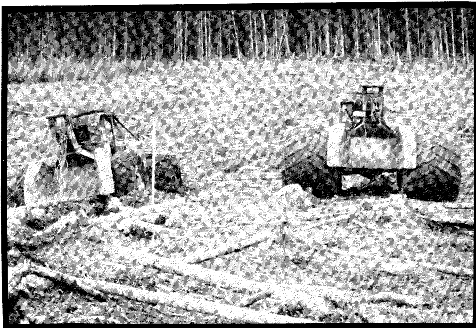
Figure 24. Slope Test Track Comparison. Note difference in ground disturbance between conventional and wide tires.
