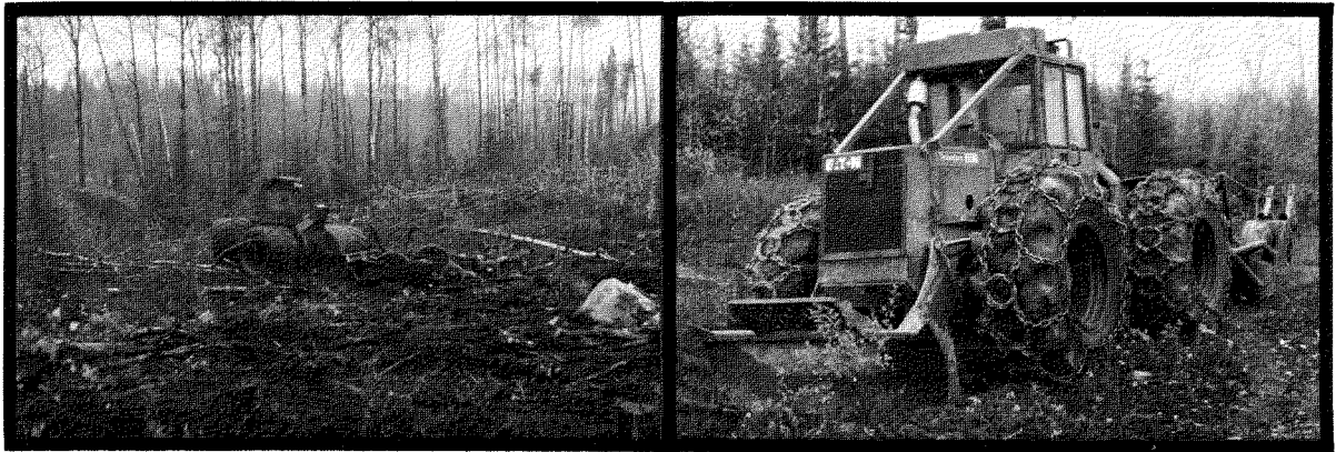
Figure 19. Scarification Test Machines. The United "Super Muskeg" tires are pictured on the left and the standard (30.5 in.) tires with chains are shown on the right.
