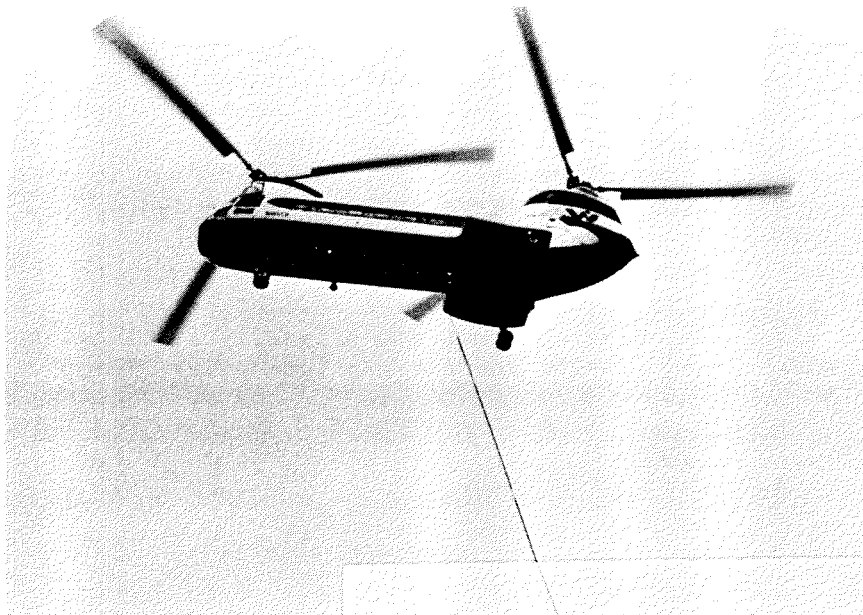
FIGURE 4. Logging with a Boeing Vertol 107.
