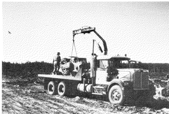
Figure 5. A machine frame is lifted onto a straight truck for transport to town for repairs.
