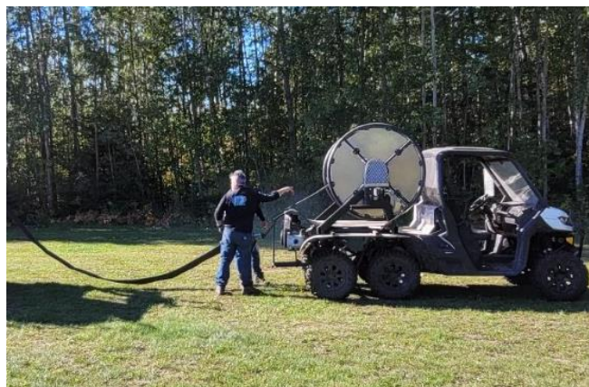
Figure 5. Hose lay done with a UTV.
