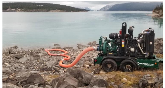
Figure 2. Large water source required. Pump site requires stable ground. Pump needs to be close to the water.
