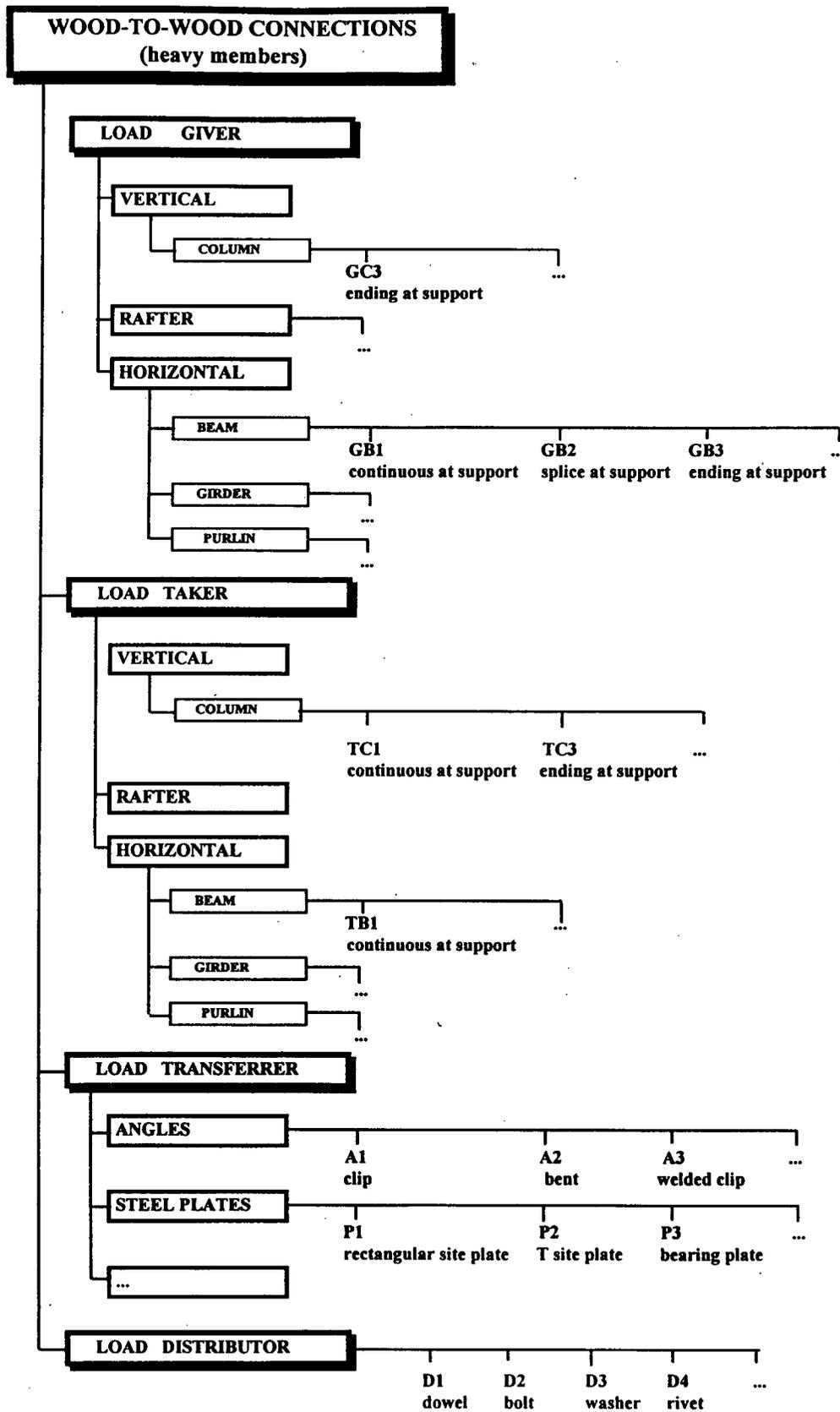
Figure 2. Key components in functional hierarchy (Varoglu *et al.* 1995).
