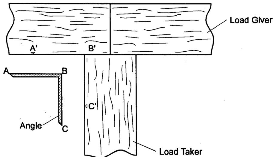
Figure 3. Shared surfaces of an angle between load giver and taker (Varoglu *et al.* 1995).
