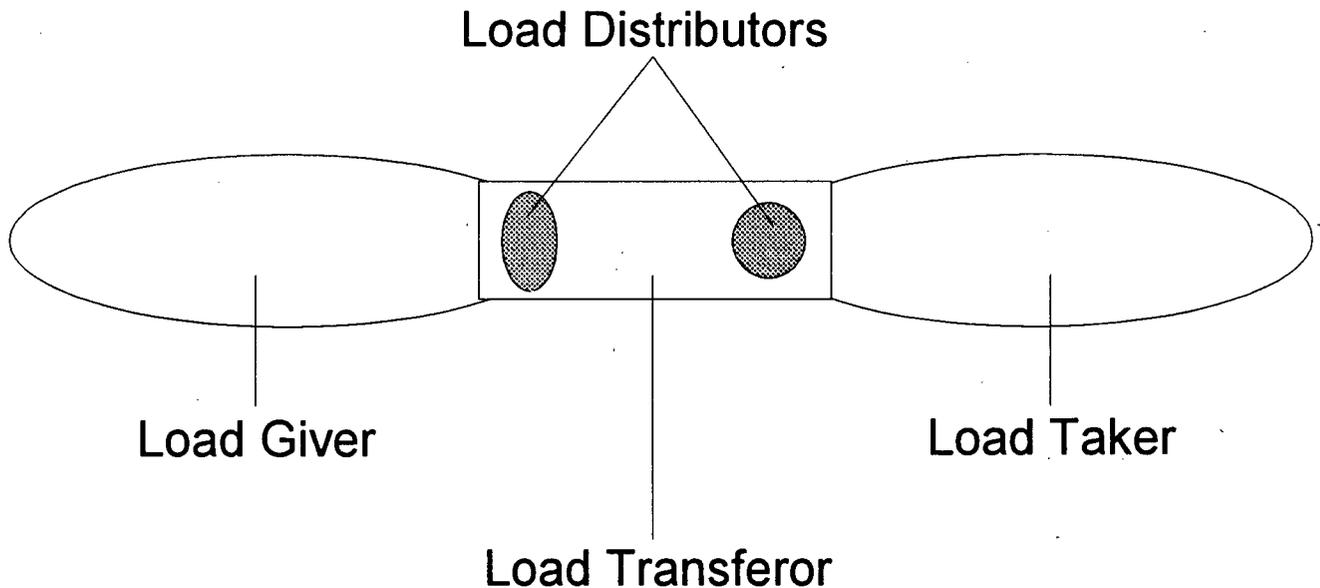
Figure 1. An abstraction of a timber connection according to the function of components.
