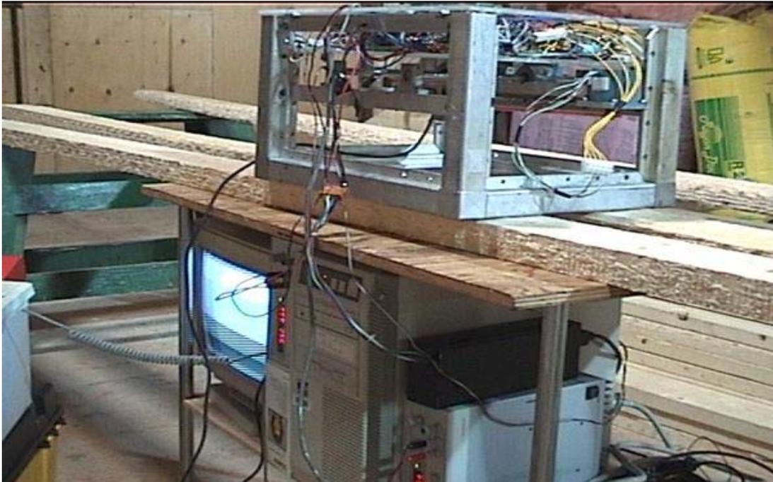
*Figure 5 Scanner for measuring knot tear-out volume*
