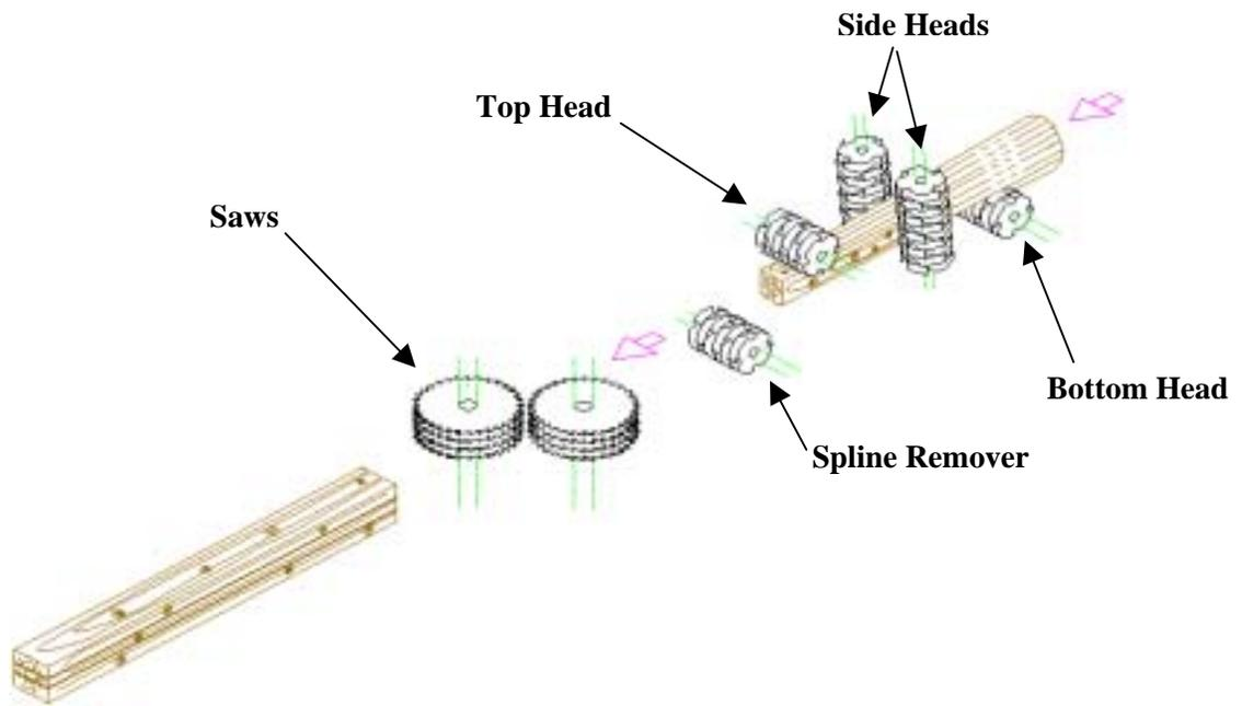
**Figure 1** *Schematic of Chipping Canter Line*
