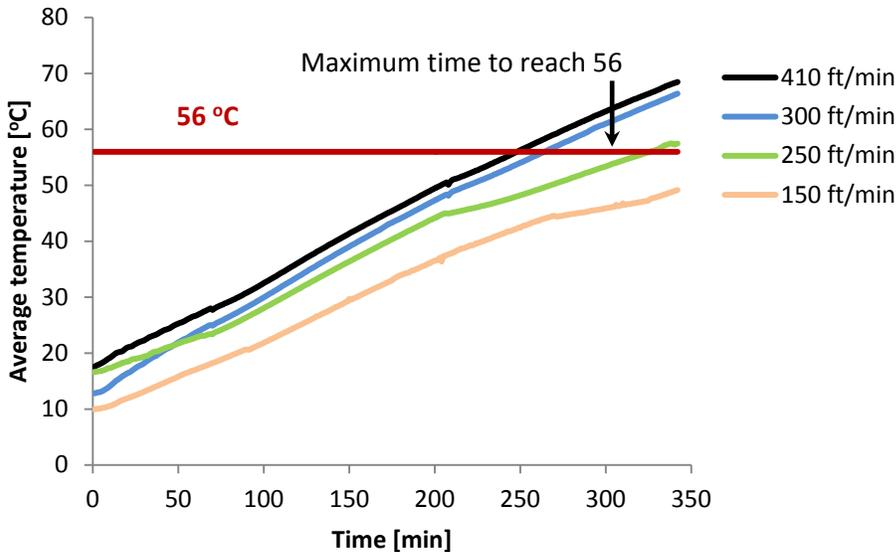
**Figure 5** Average temperature increase for different air velocities
