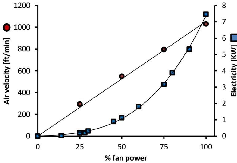
**Figure 4** The relationship between air velocity and electricity consumption
