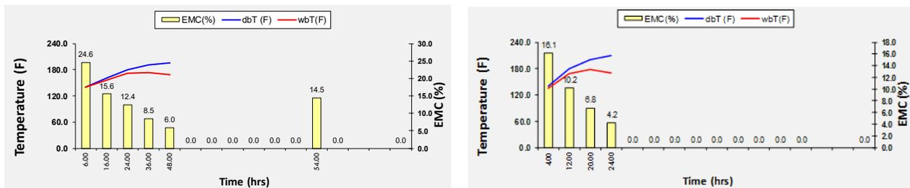
Figure 1 Drying parameters in a conservative (left) and an accelerated drying schedule for SPF
