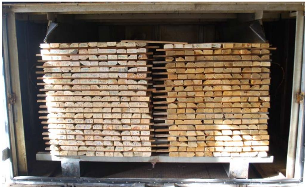
**Figure 2** Front view of the fully loaded kiln before a HT test
