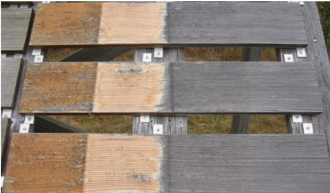
Figure 5 Samples with no Pre-Treatment after 24 months exposure
