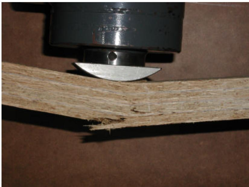
**Figure 4: Typical failure mode for a 4-ply specimen (Tension failure of bottom and centre laminations)**
