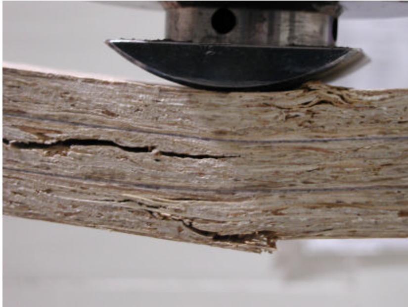
**Figure 3: Detail: Typical failure mode for a 3-ply specimen [Tension failure (bottom lamination), shear failure (centre lamination), localized compression (top lamination)]**
