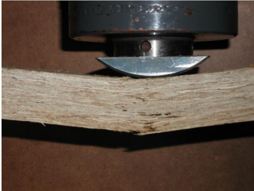
**Figure 1: Typical failure mode of control specimens (Tension failure)**
