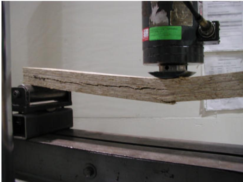
**Figure 2: Typical failure mode for a 3-ply specimen (Shear failure through centre lamination)**
