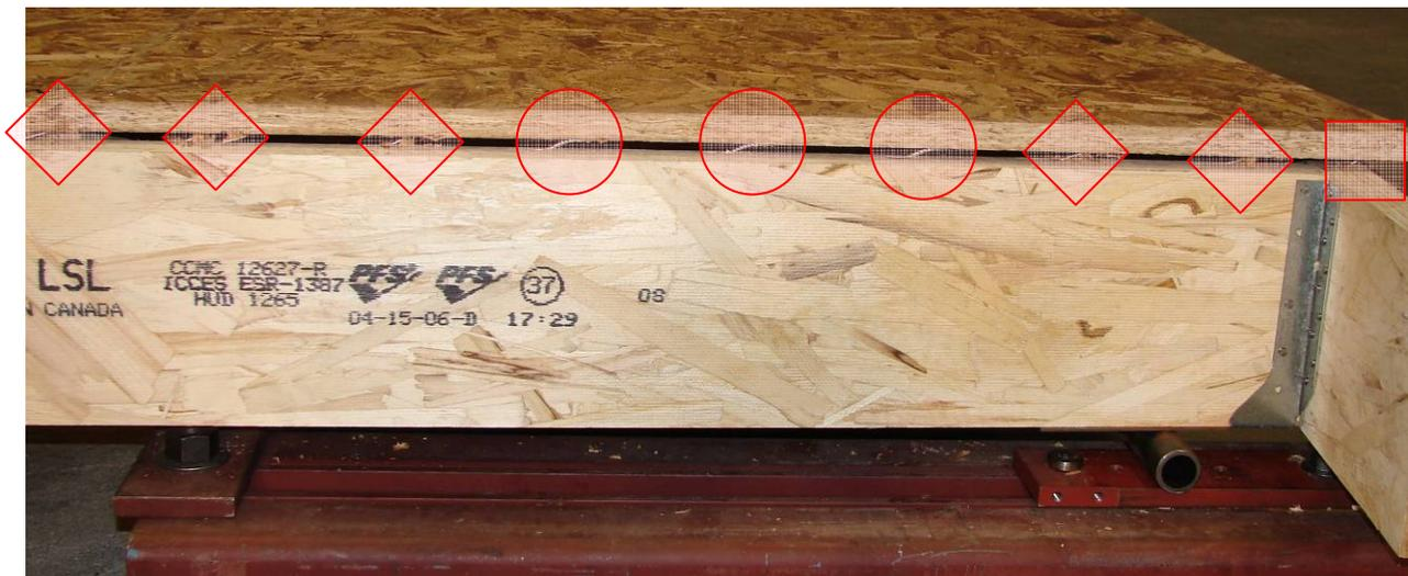
**Figure 7: Detail of failed sheathing-to-framing connection in diaphragm D9 (Legend for shapes: diamond – nail pull through, circle – nail withdrawal, square – nail fatigue)**
