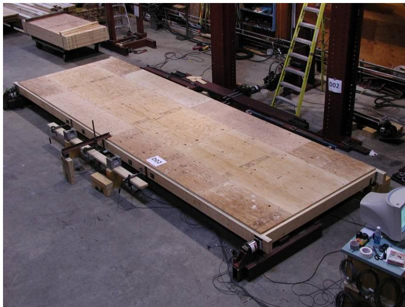
**Figure 1: Example of a diaphragm constructed with double SPF framing and plywood sheathing (diaphragm D2)**
