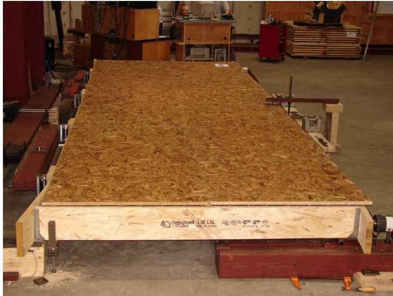
**Figure 6: Characteristic failure mode of a diaphragm constructed with LSL framing and OSB sheathing (diaphragm D9)**
