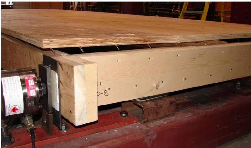
***Figure 5: Detail of the diaphragm side that failed due to nail withdrawal (diaphragm D2)***
