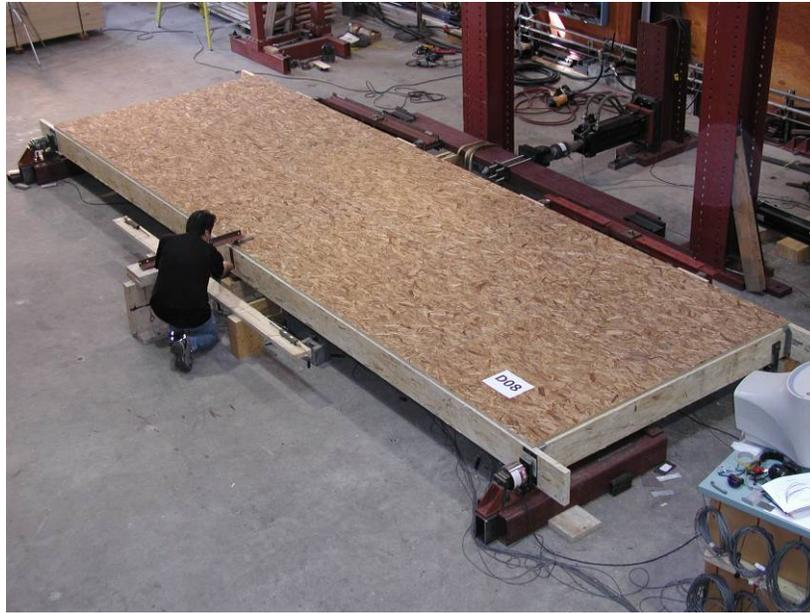
**Figure 2: Example of a diaphragm constructed with TimberStrand® LSL framing and OSB sheathing (diaphragm D8)**
