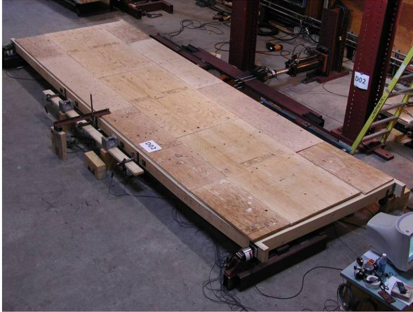
***Figure 4: Characteristic failure mode of a diaphragm constructed with double SPF framing and plywood sheathing (diaphragm D2)***
