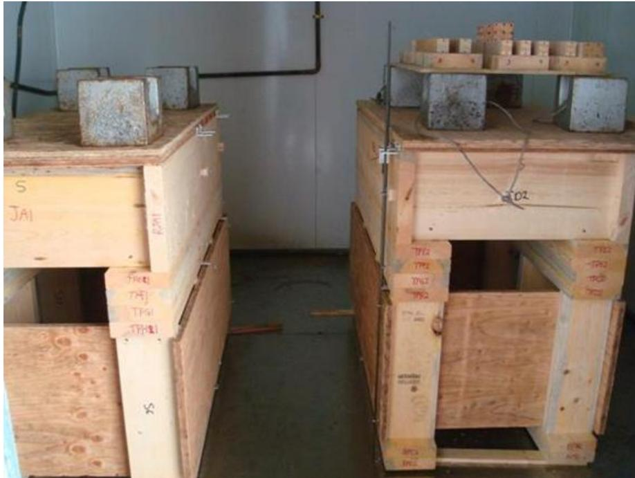
**Figure 2** *Conditioning the two structures under a small load in a conditioning chamber*
