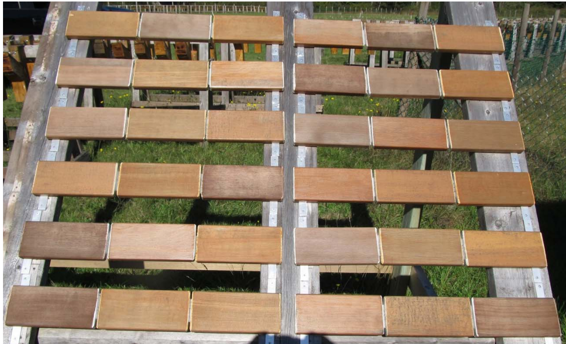
Figure 1 Photograph of Samples after Six Months' Exposure in Maple Ridge, BC
