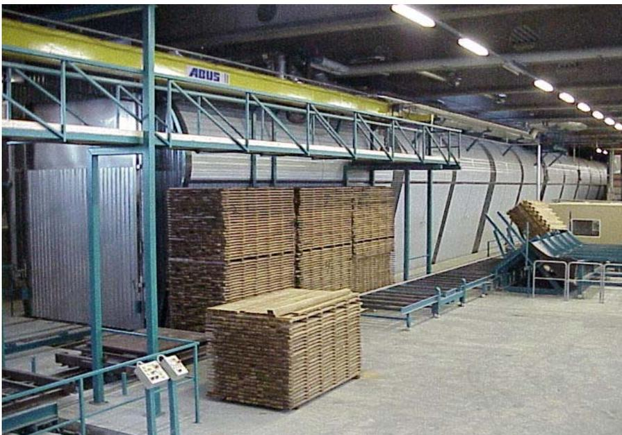
**Figure 3: Thermo Wood Continuous Through Feed Treatment Facility**
