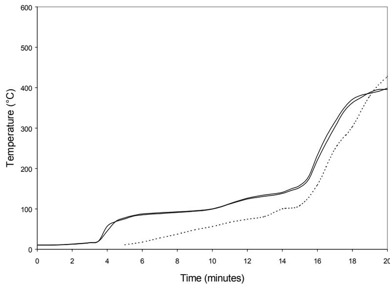
Figure 5. Comparison of predicted and measured temperatures within a wall in Test 2.
