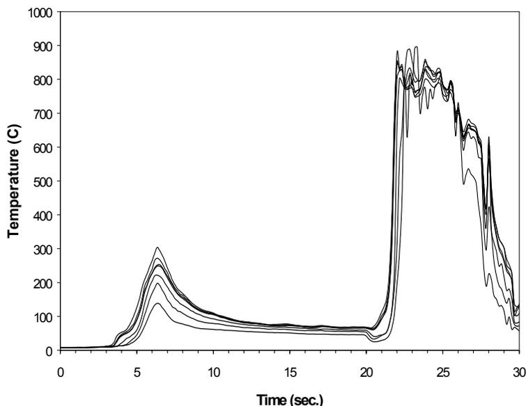
**Figure 3** *Temperatures measured in fire in a basement recreation room*
