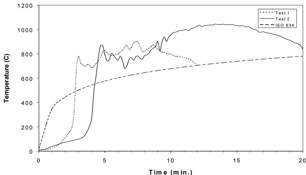
Figure 2. Temperatures in Tests 1 and 2 compared to the ISO 834 curve.
