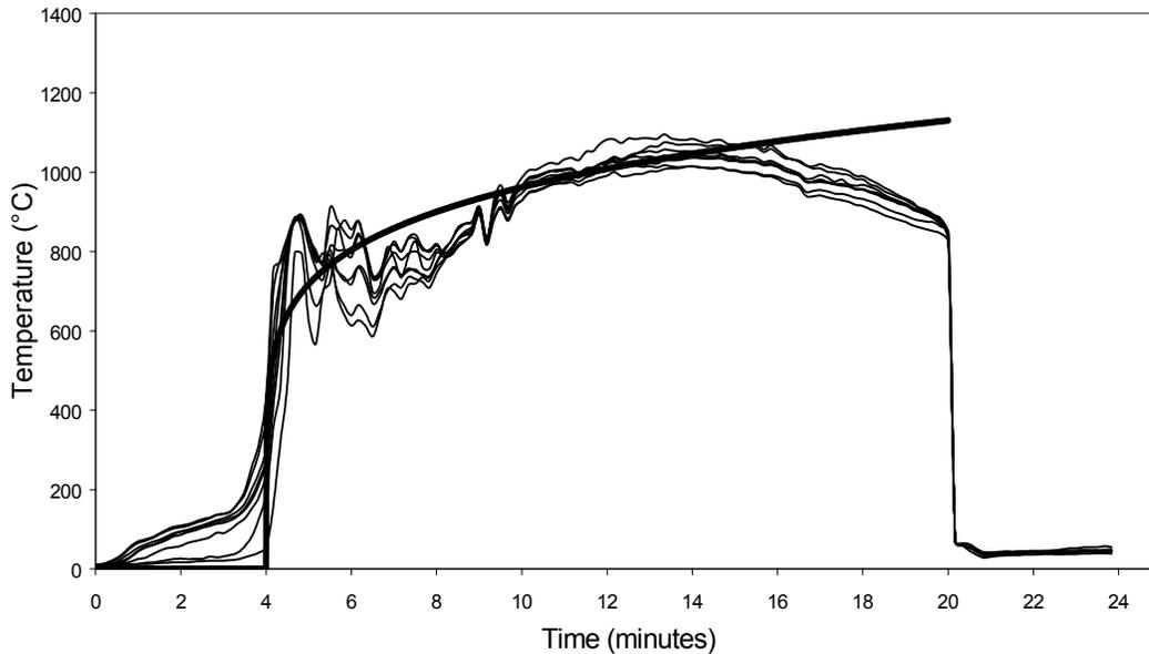
Figure 4. Fit of  $\Delta T_h = \beta t^{1/6}$  ( $\beta = 355$ ) to the temperature data of Test 2.
