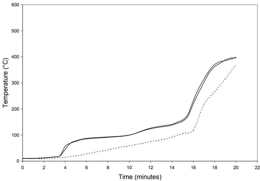
Figure 5: Comparison of predicted and measured temperatures within a wall in Test 2.
