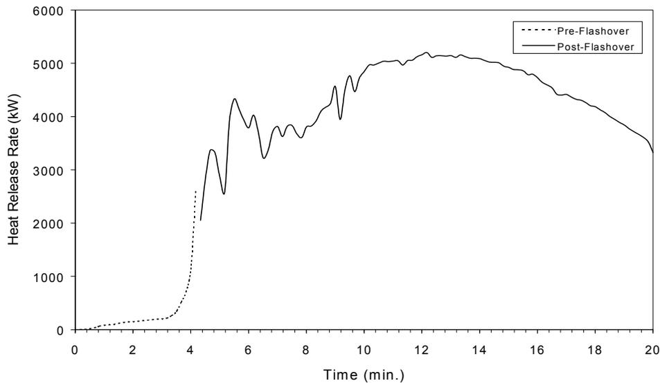
Figure 3. An estimate of the heat release rate during Test 2
