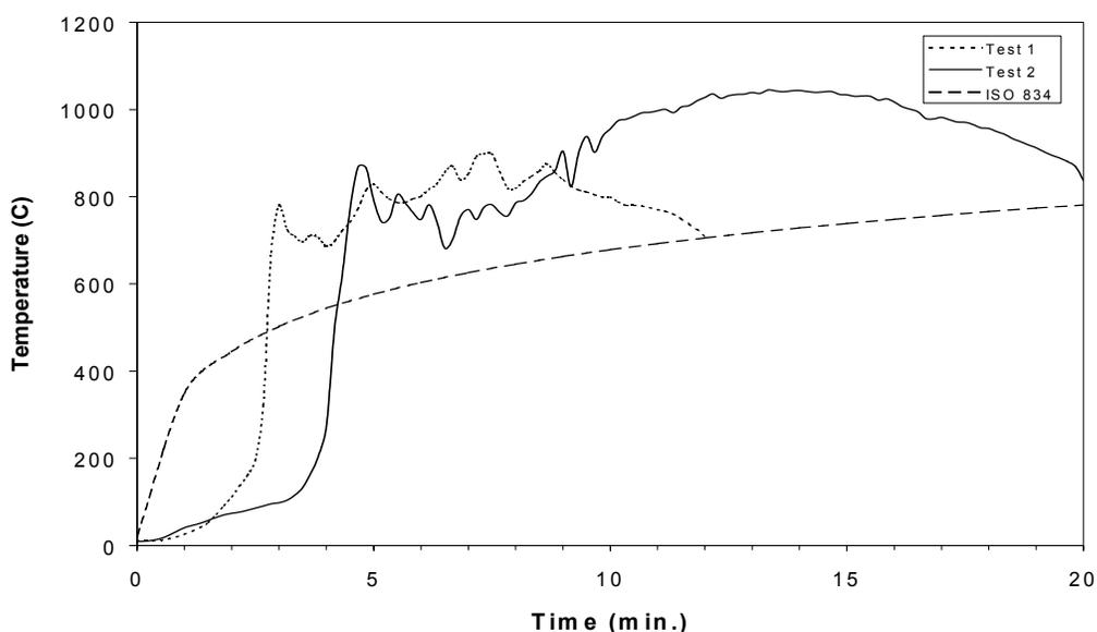
Figure 2. Temperatures in Tests 1 and 2 compared to the ISO 834 time-temperature curve.
