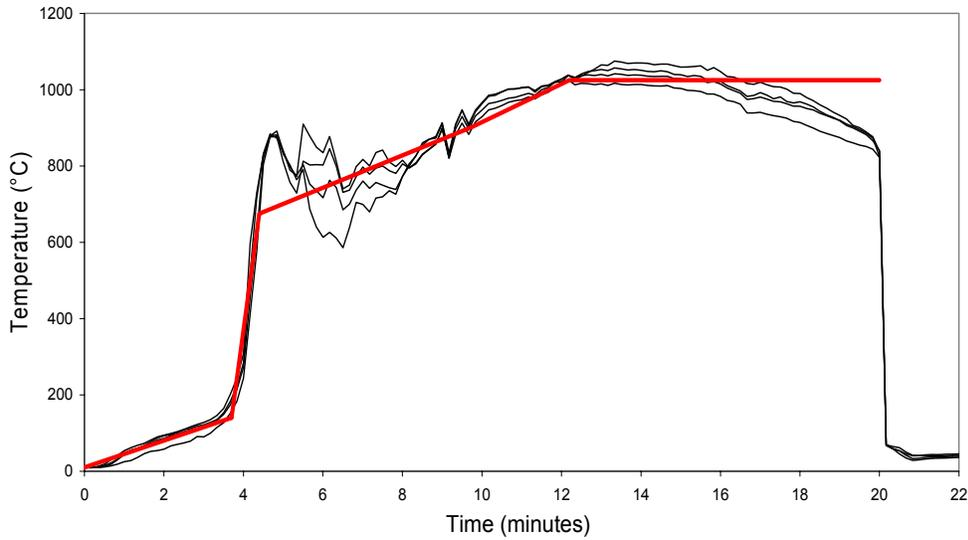
**Figure 1** *Approximation of the fire temperature measured in Test 2*
