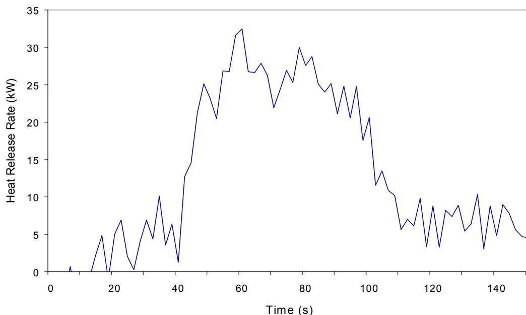
Figure 1: The Heat Release Rate of the Waste-paper Basket Fire
