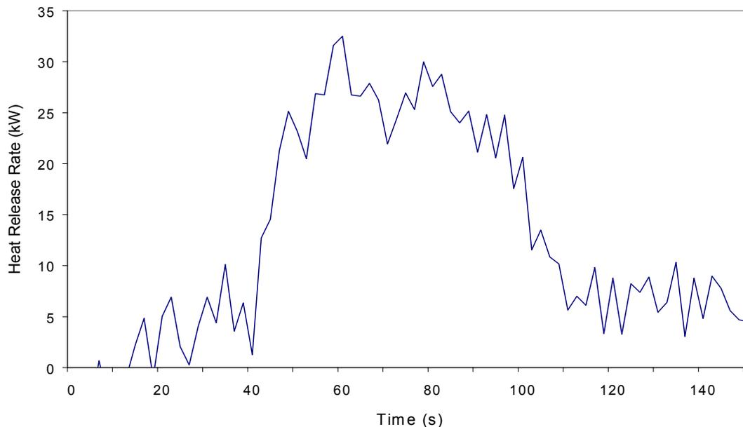
Figure 1. The heat release rate of the waste-paper basket fire
