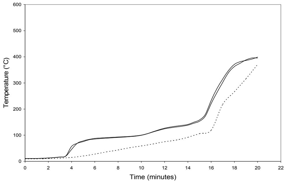
**Figure 2** *Comparison of predicted and measured temperatures within a wall in Test 2*
