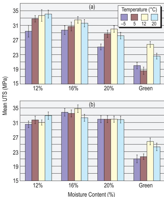
Figure 1. Effect of moisture content and temperature on the UTS for: (a) PEP; (b) PRF adhesives
