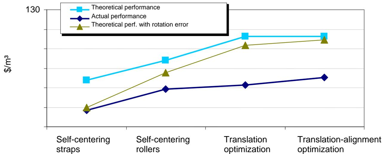
**Figure 13 Impact of rotation errors with the different infeed types**
