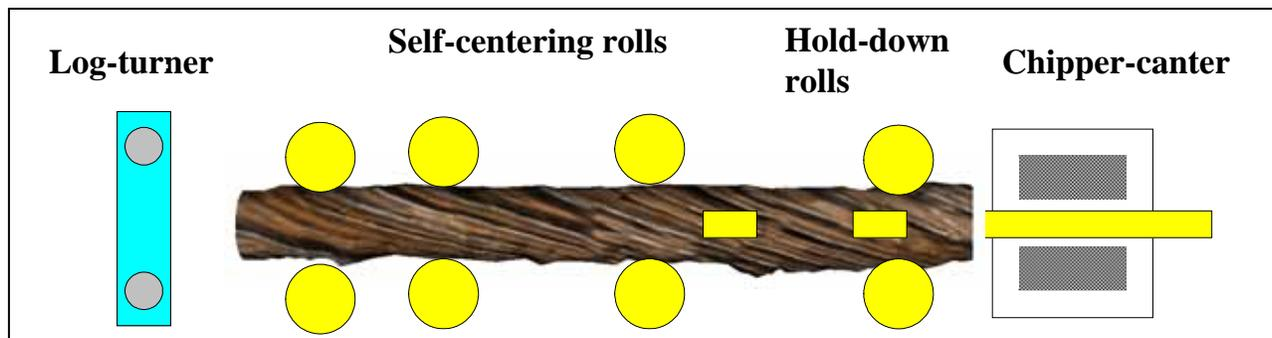
**Figure 3 Self-centering roller device**
