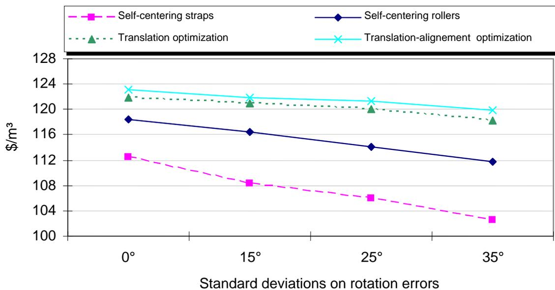
**Figure 14 Impact of rotation errors on value recovery**
