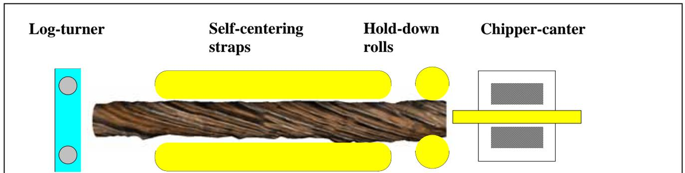
**Figure 2** *Self-centering device*
