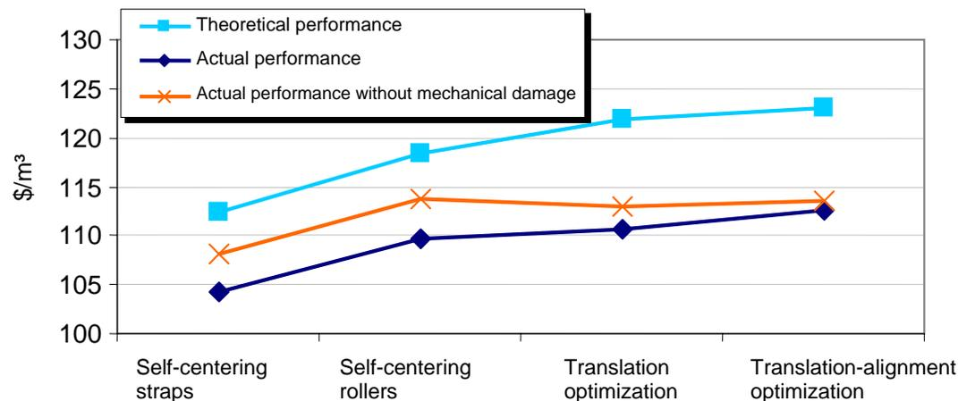
**Figure 12 Value recovery from simulations based on logs, cants and filtered cants**
