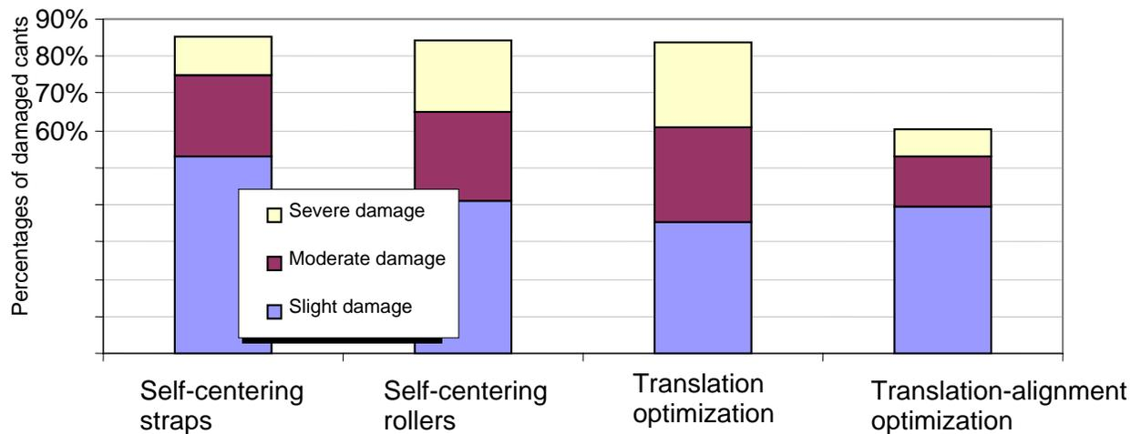
**Figure 10 Percentages of cants showing mechanical damage**
