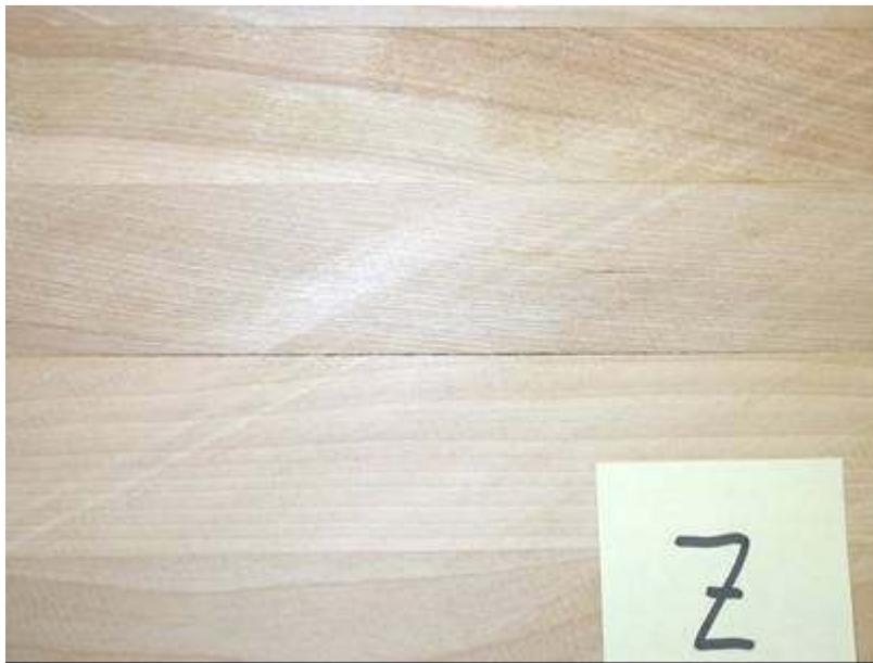
**Figure 13** *Apparent glue line: uneven saw kerf straightness; max. opening 0.79 mm*
