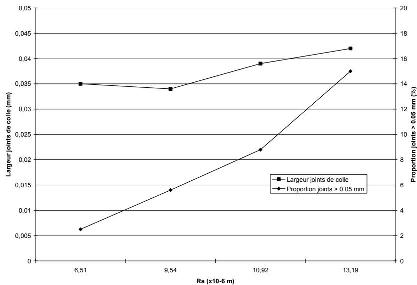
**Figure 29** Average glueline width and proportion of gluelines >0.05 mm with relation to R<sub>a</sub>
