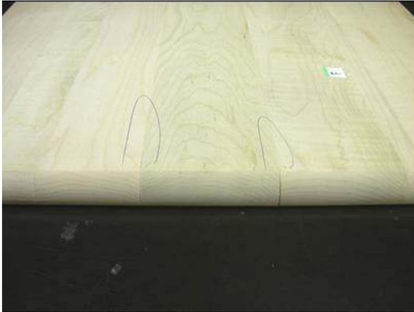
**Figure 14** *Apparent gluelines: open-end gluelines*
