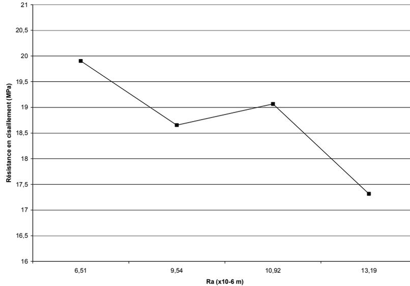
**Figure 17** *Glueline shear strength in relation to  $R_a$*
