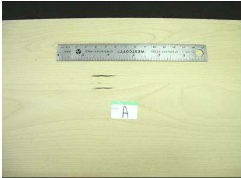
**Figure 8** *Apparent glueline: splintering of the edge, 0.6 mm cavity*
