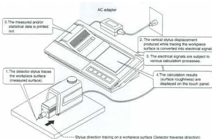
Figure 2 Stylus probe profilometer
