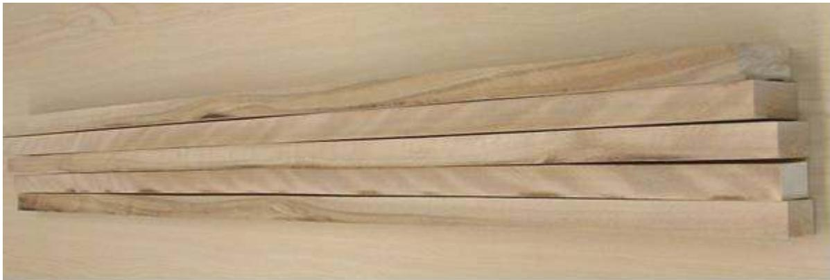
**Figure 15** Edges of strips ripped with used saw blades
