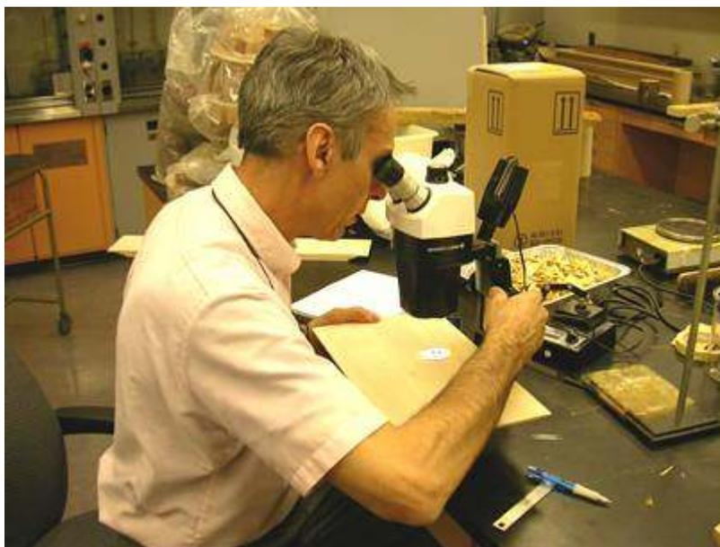
***Figure 1*** Microscopic measurement of glueline width
