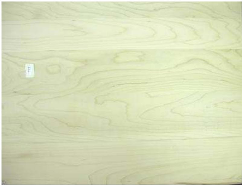
**Figure 10** *Apparent gluelines: excessive edge roughness or insufficient clamp pressure; glueline width 0.07 to 0.15 mm*
