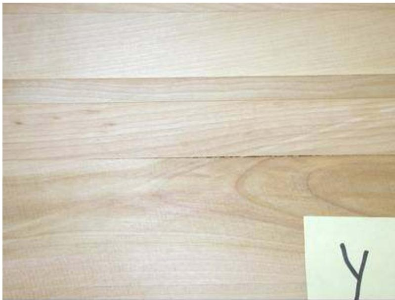
**Figure 12** *Apparent glueline: uneven saw kerf straightness; max. opening 0.82 mm*
