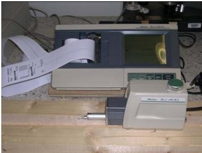
**Figure 6** *Measuring edge roughness with the stylus probe profilometer*
