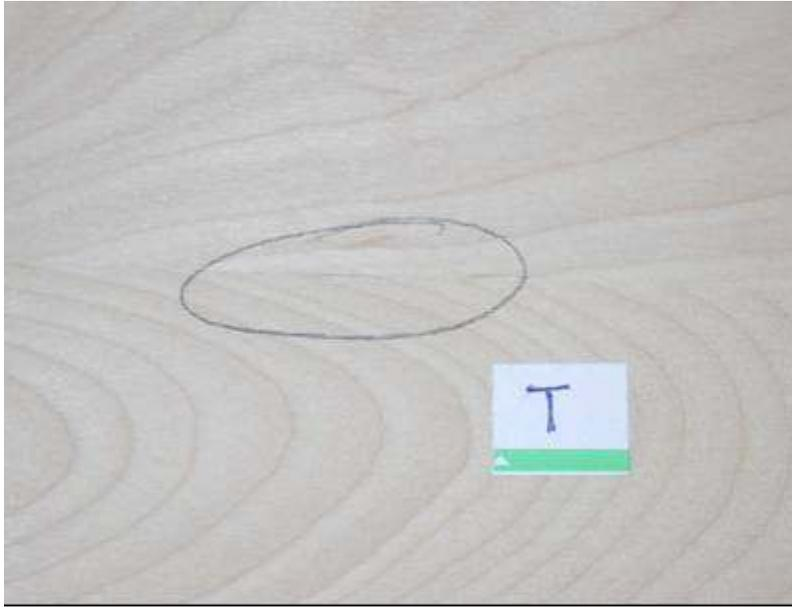
**Figure 9** *Apparent glueline: splintering of the edge; 0.08 mm cavity*
