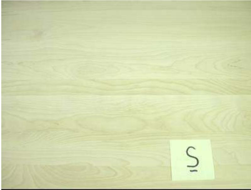
**Figure 11** *Apparent gluelines: excessive edge roughness or insufficient clamp pressure; glueline width 0.08 mm*
