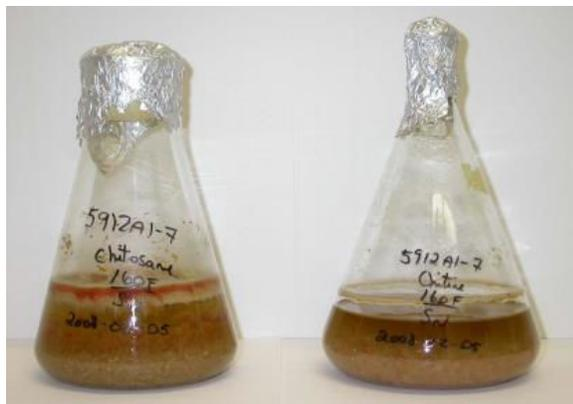
**Figure 2. Fungal modification of chitosan by a fermentation process**
