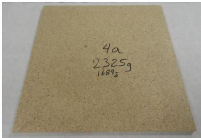
Figure 26. Particleboard made with 1% chitosan resin and 66% UF resin in 1:1 ratio
