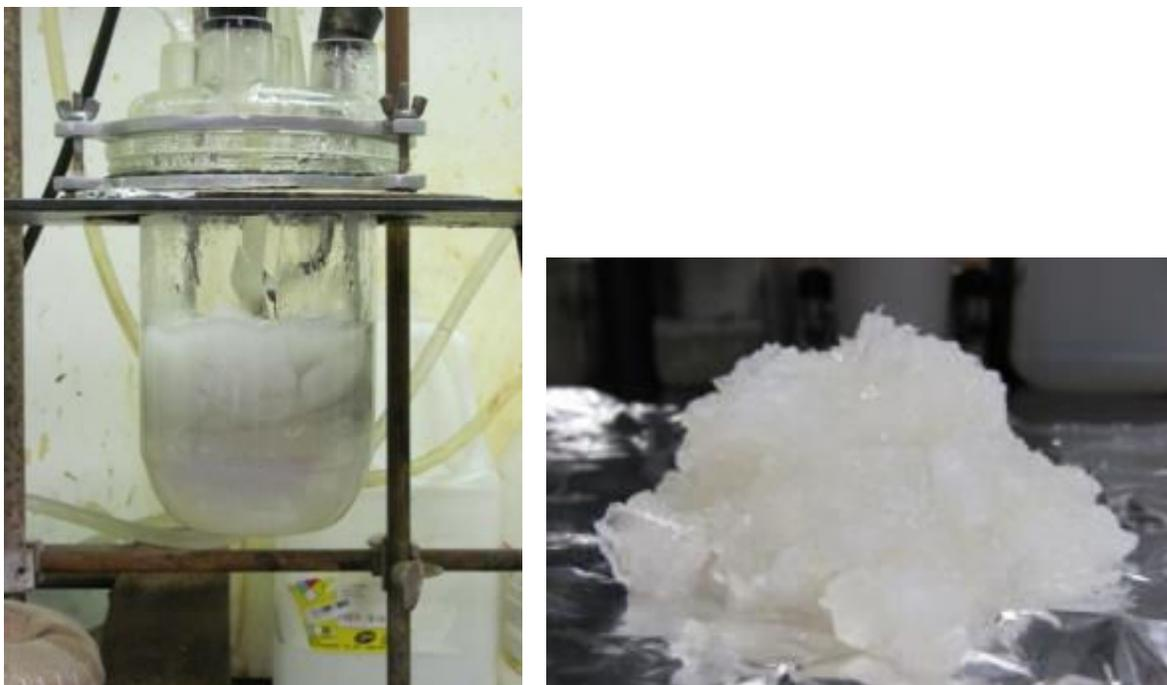
**Figure 21. Gelation of unmodified chitosan solution with the mixture of formaldehyde and urea at an early stage of the UF synthesis process**
