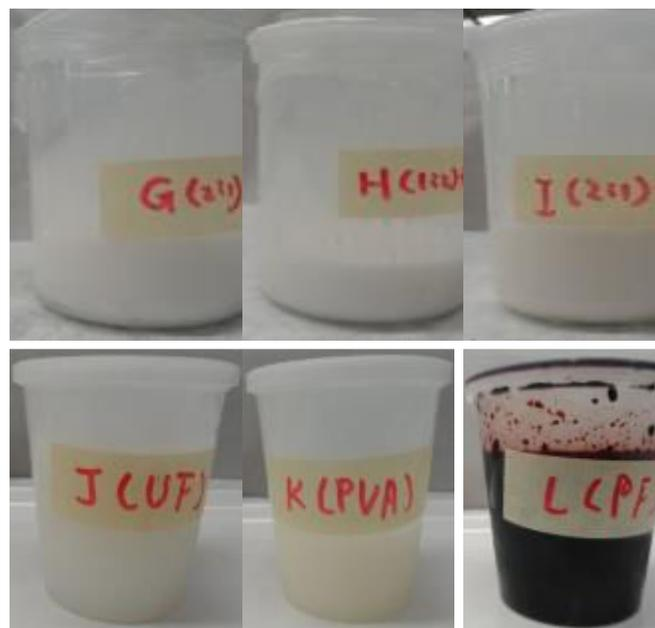
Figure 10. Appearance of three chitosan-based resins G to I and three commercial resins J to L
