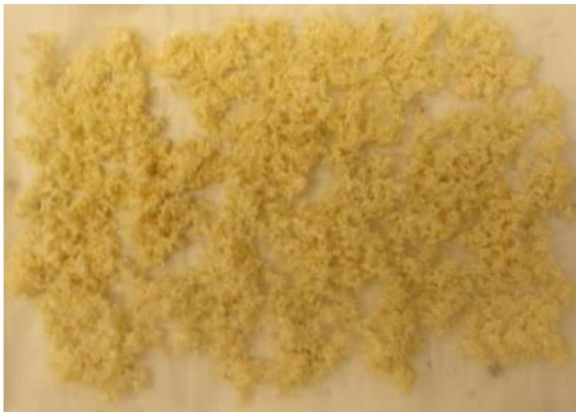
**Figure 6.** Chitosan modified by enzyme extracted from fungal strain 321U
