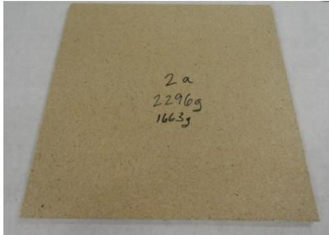
Figure 25. Particleboard made with 1% chitosan adhesive
