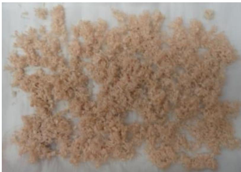
**Figure 7.** Chitosan modified by enzyme extracted from fungal strain 161D
