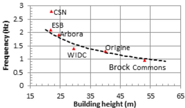
Figure 3. Results of AVT in comparison of the NBCC equation
