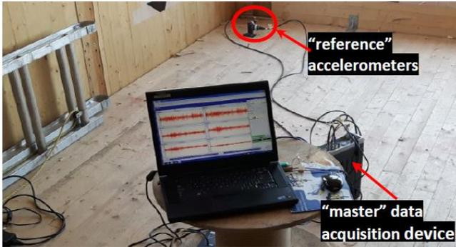
Figure 2. AVT measurement being performed at the Origine building in Quebec City
