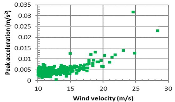
Figure 4. Peak acceleration response measured for different wind velocity for the Arbora building in Montreal
