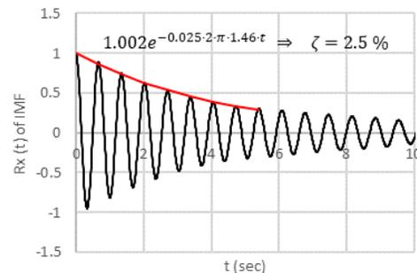
Figure 5. Extraction of the damping ratio with autocorrelation function from the TVF-EMD algorithm
