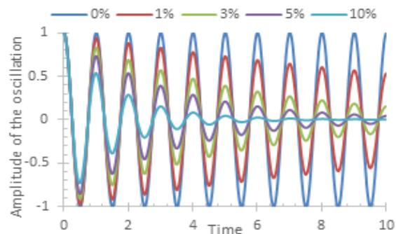
Figure 1. Decay of a free oscillation for different damping ratios
