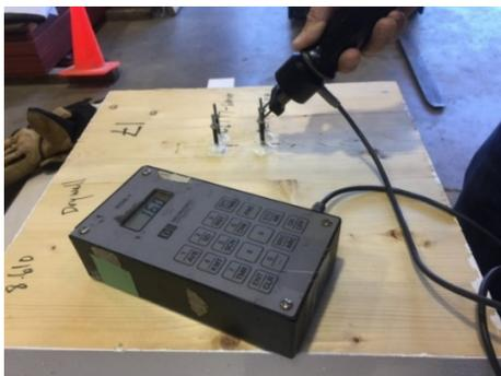
Figure 2. Measuring wood moisture content using a portable pin moisture meter (top) and pre-installed moisture pins (bottom).
