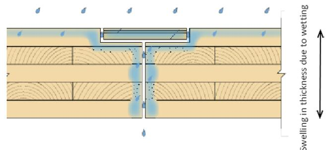
Figure 1. Potential for water absorption at end grain and splines between CLT panels; swelling in the thickness direction.
