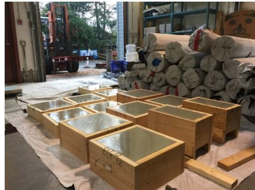
Figure 1. Wood specimens with their top surfaces covered with wet light-weight self-leveling concrete using pre-built forming.
