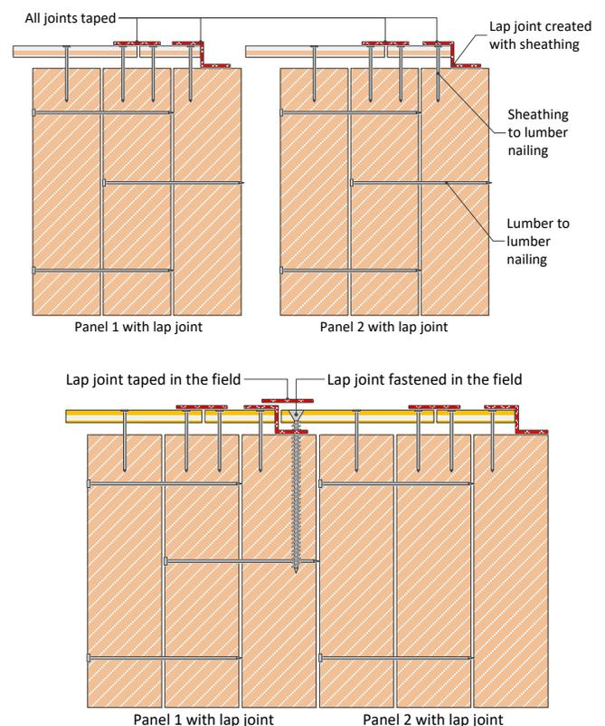
Figure 4. Basic Option 1: for a low wetting risk environment, pre-sealing all joints between sheathing in factory (above), and re-sealing lap joints at job site (below).
