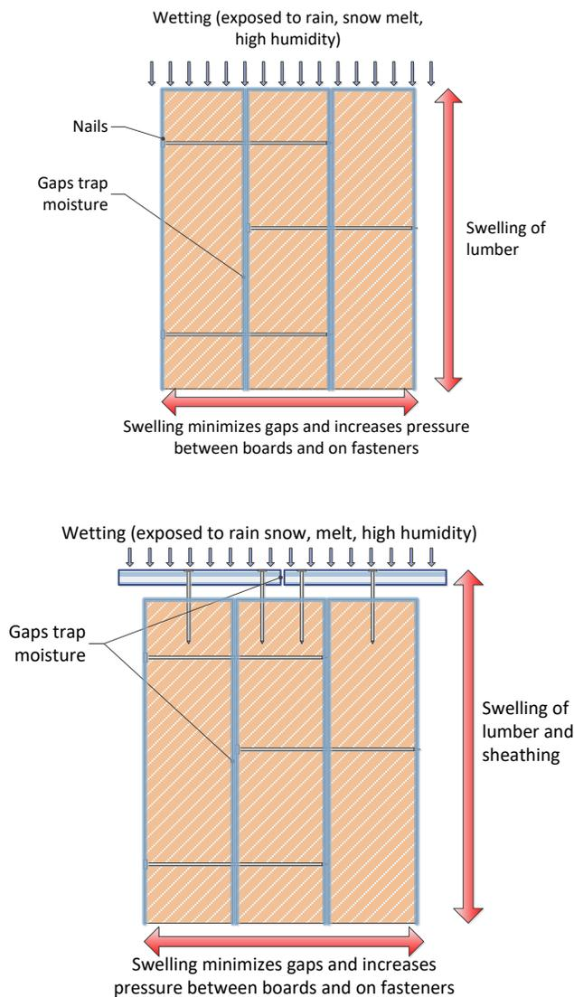
Figure 2. Potential of trapping water between boards of NLT and between NLT and sheathing, and potential swelling resulting from wetting (top: NLT; bottom: NLT with sheathing. Blue indicates wetting for an illustrative purpose).
