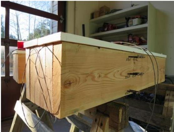
Figure 3. Measuring wood moisture content using a portable pin meter (top) and pre-installed moisture pins (bottom).
