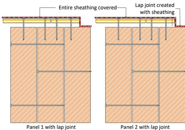
Figure 5. Basic Option 2: for a moderate level of wetting risk, pre-protecting entire sheathing in factory, and re-sealing lap joints at job site.
