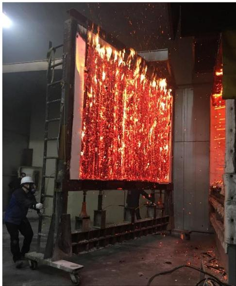
Figure 3. End of a DLT wall fire resistance test
