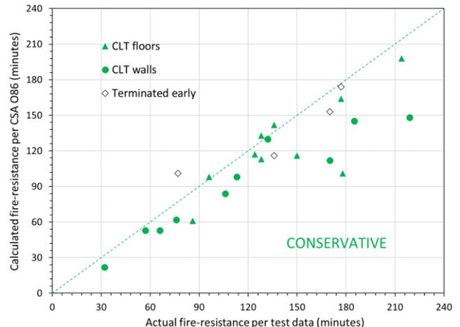
Figure 2. Calculated CLT fire resistance vs. test data
