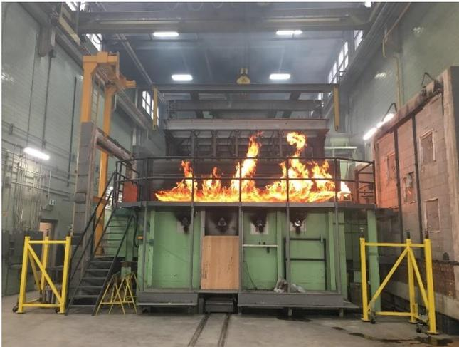
Figure 1. Removal of a GLT floor after a FPIinnovations fire resistance test conducted at National Research Council Canada
