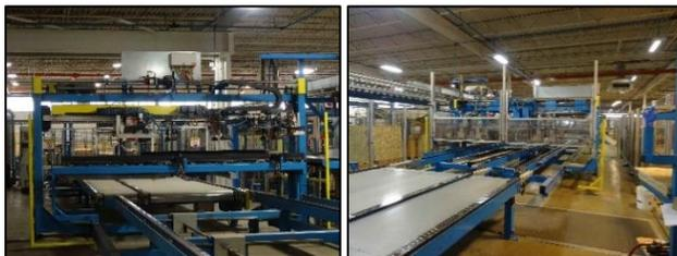
Figures 5 and 6. Automated panelized production line (Courtesy: H+ME Technology)
