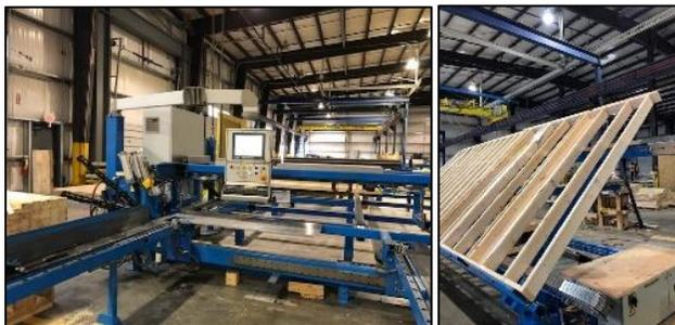
Figures 5 and 6. Semi-automated panelized line (Courtesy: ZyTech Building Systems)
