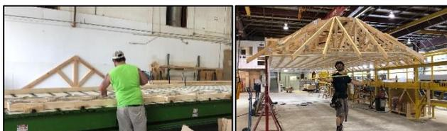
*Figure 1. Truss manufacturing (Courtesy: Royal Homes)*      *Figure 2. Roof truss system (Courtesy: Quality Homes)*
